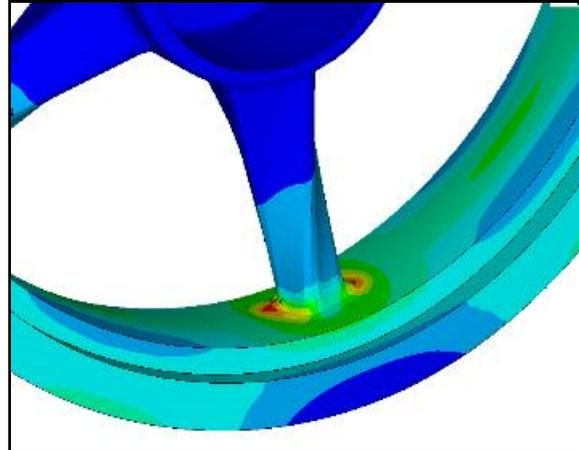
Fig 8: Zoom in view von-Mises Stress Plot
