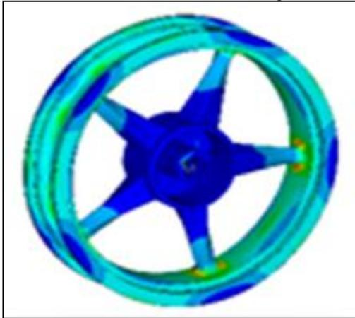
Fig 7: Maximum von-Mises Stress Plot
