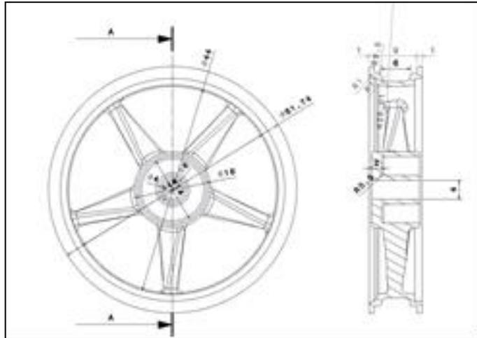
Fig 2: Geometry of the 5 spokes wheel.
