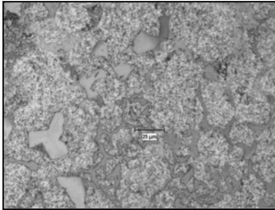
Fig 6: 1mm & 60 Gm SiO<sub>2</sub> (Killer's Etched 500X).
