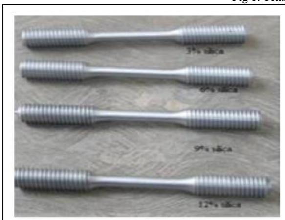
Fig 2: Tensile Specimen before Test.
