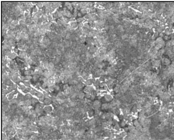
Fig 9: 3mm & 60 gm SiO<sub>2</sub> (Unetched-100X).
