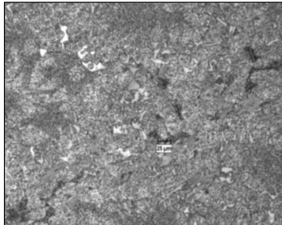
Fig 8: 5mm & 60 gm SiO<sub>2</sub> (Killer's Etched 500X).
