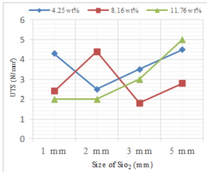
Fig 11: Plot of UTS v/s Size of Silica.
