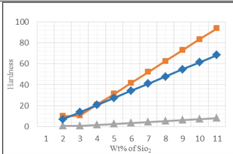
Fig 12: Hardness v/s wt. % of Silica.
