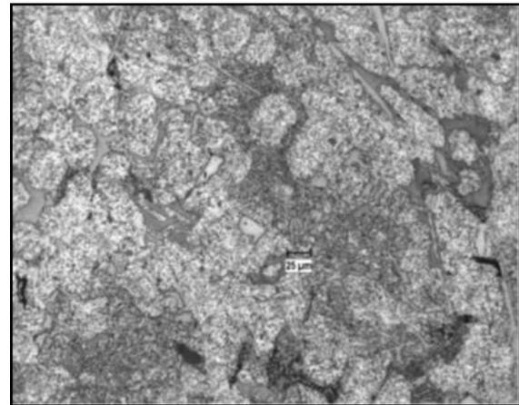
Fig 10: 3mm & 60 gm SiO<sub>2</sub> (Killer's Etched 500X).
