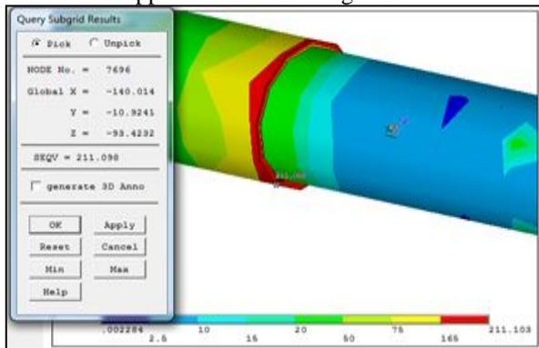
Fig 15: Query Results for Node at Max Stress.
