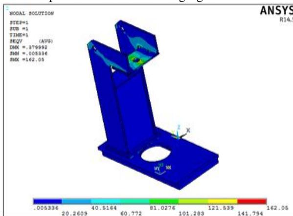
Fig 10: von-Mises Stresses in Base Plate.
