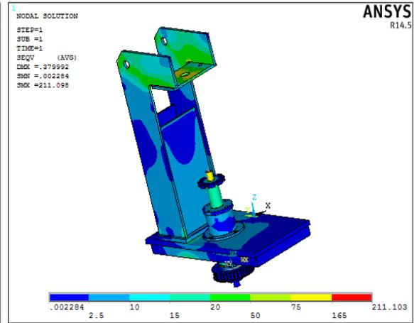
Fig 9: Von-Mises Stress Plot.
