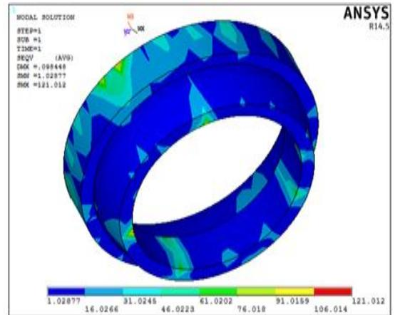
Fig 11: von-Mises Stresses in Gland
