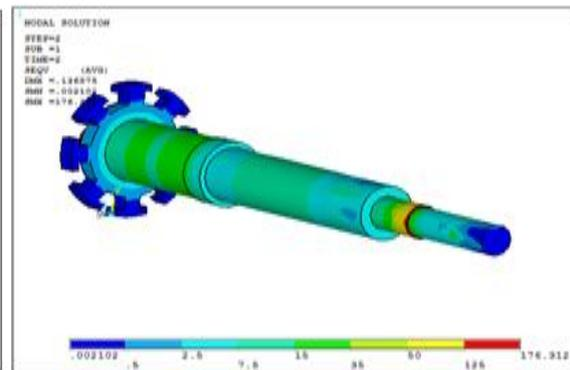
Fig 18: Stress with the Crack for 90000N-mm Torque.
