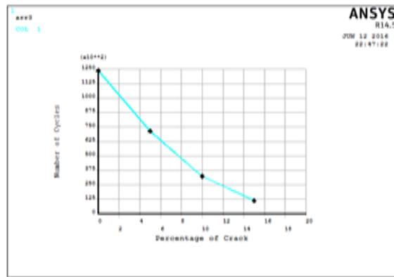
Fig 20: Percentage of Crack vs. Number of Cycles.
