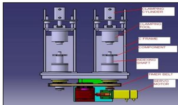
Fig 4: Complete representation of the Assembly.
