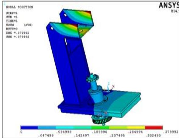
Fig 8: Displacement Plot of Assembly
