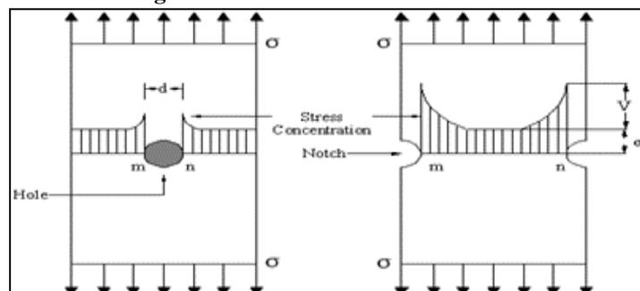
Fig 1: Stress Concentration due to Cutouts.
