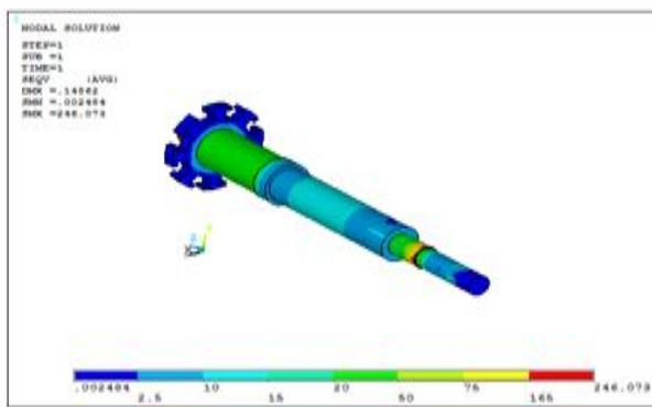
Fig 17: Stress for 120000N-mm Torque
