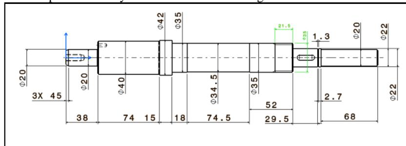
Fig 6: Dimensional view of the Spindle Shaft
