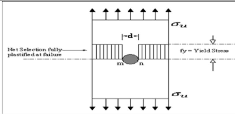
Fig 2: Stress reaching to Yield Stress at the Cut-out.
