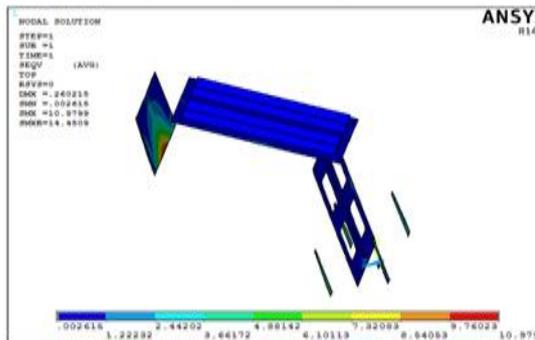
Fig 17: von-Mises Stress in 12mm sections.
