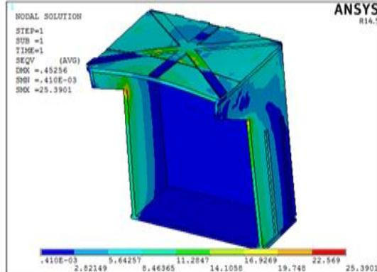
Fig 10: von-Mises Stress Plot.
