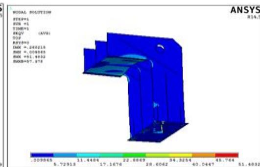
Fig 18: von-Mises Stress in 20mm Sections.
