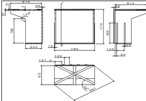
Fig 2: Dimensional Representation of the C-Press (Model 1).
