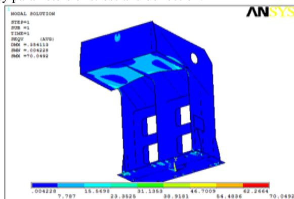
Fig 21: Von-mises Stress plot for the final optimized set.
