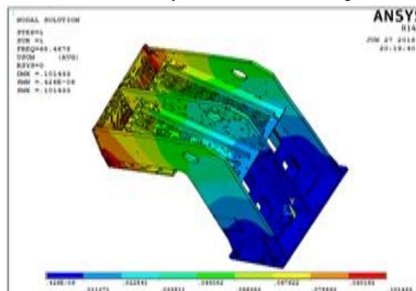
Fig 19: Mode Shape for the Conceptual design 2.
