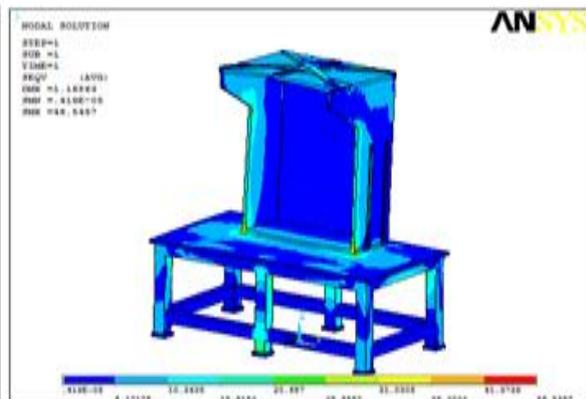
Fig 14: von-Mises Stress Plot.
