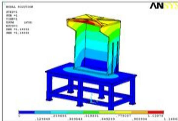
Fig 13: Displacement plot.
