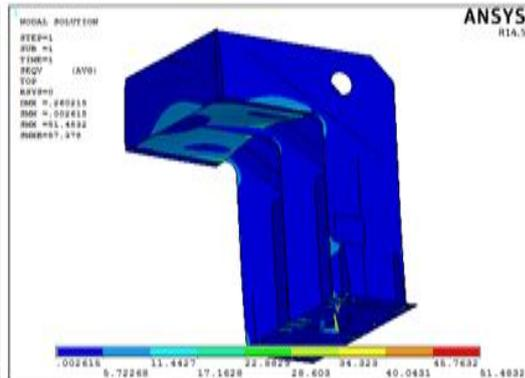
Fig 16: von-Mises Stress Plot.
