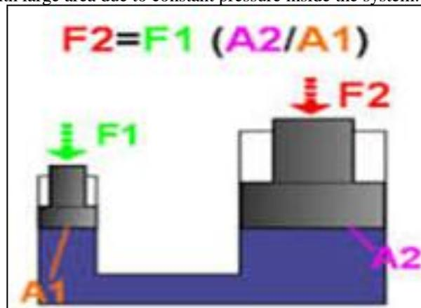
Fig 1: Bramah Press Principle.
