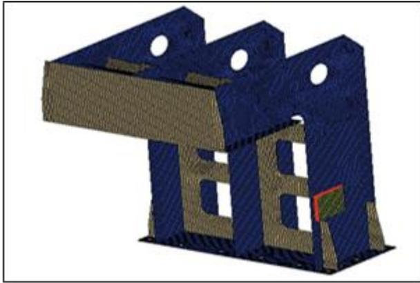
Fig 7: Mesh of the Second Conceptual Design.
