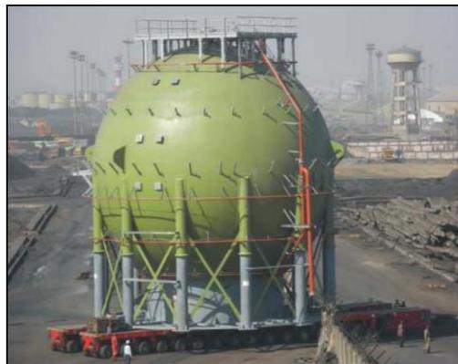
Fig 3: Spherical Pressure Vessel.
