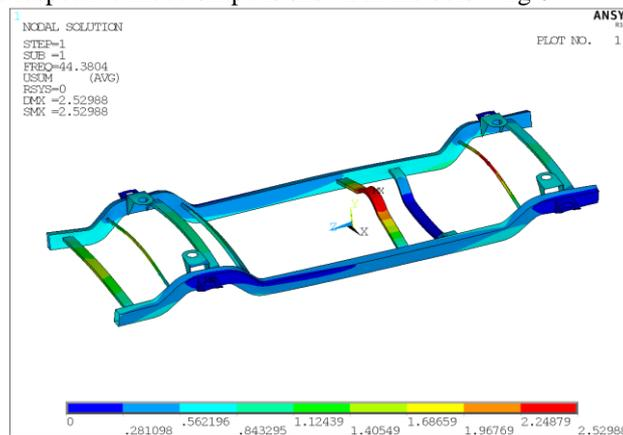
Fig 8: 1<sup>st</sup> Mode Shape with Frequency 44.38 Hz.
