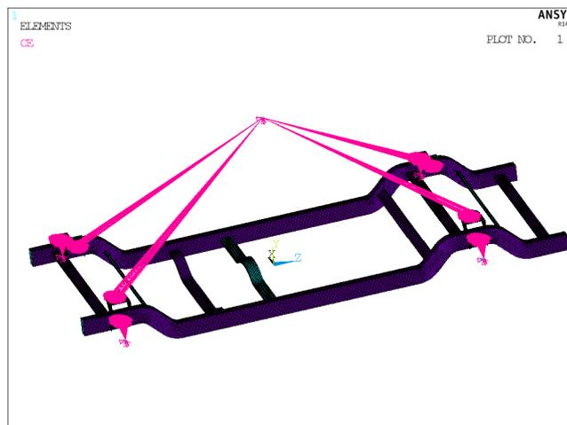
Fig 6: FE model of Car Frame.
