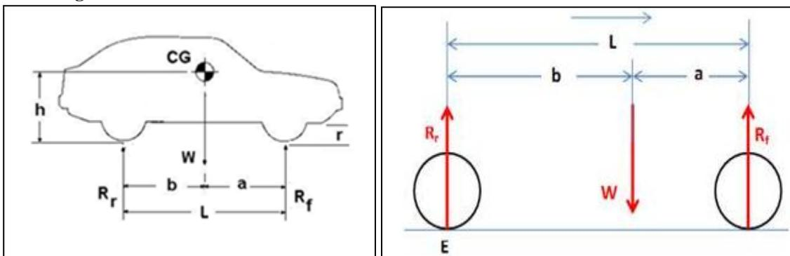
Fig 2: The CG Location in the Side View.
