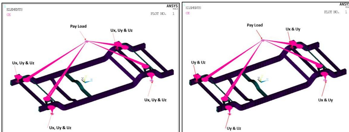
Fig 7: Boundary Conditions used in Modal and Structural Analysis.
