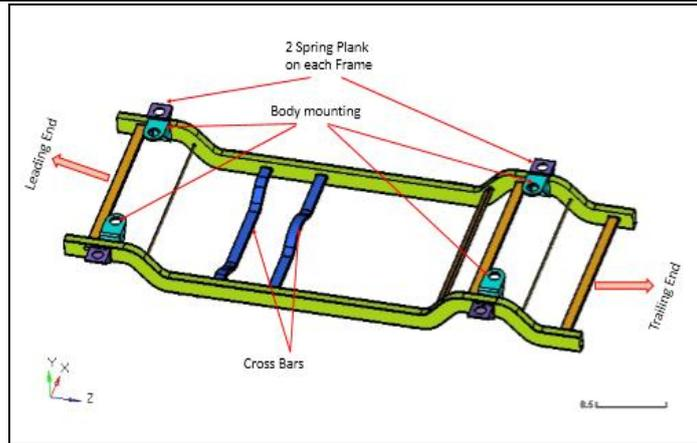
Fig 5: Geometry of the Wave Type Chassis.
