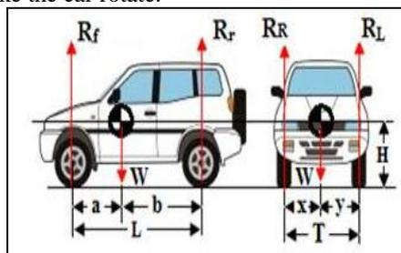
Fig 1: The CG location in the Side and Front View.
