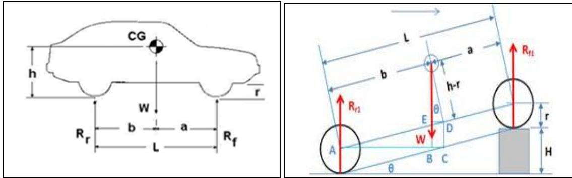
Fig 4: h is the Unknown Distance of the CG Height.
