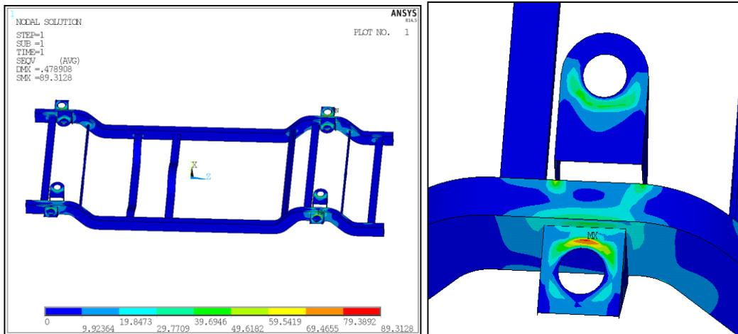
Fig 10: Maximum von-Mises Stress with Zoom in View Plots.
