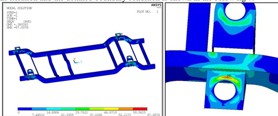
Fig 9: Maximum von-Mises Stress with Zoom in View Plots.
