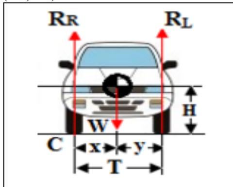
Fig 3: The CG position in the frontal view.
