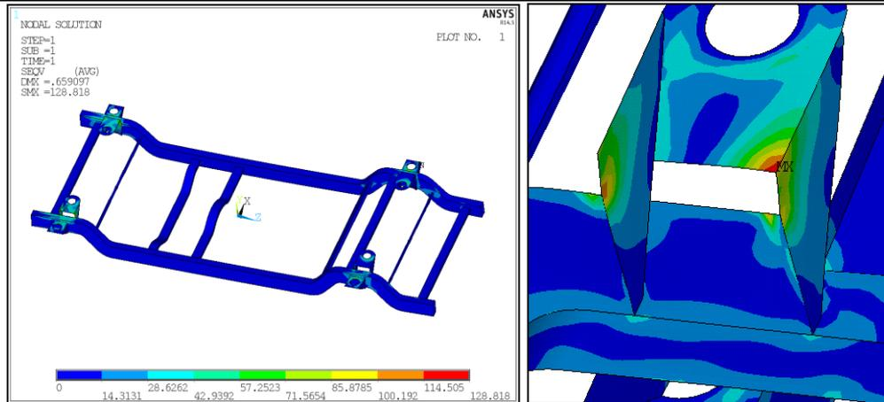
Fig 12: Maximum von-Mises Stress with Zoom in View Plots.
