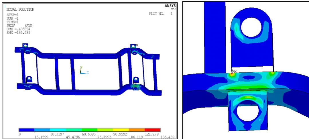
Fig 11: Maximum von-Mises Stress with Zoom in View Plots.
