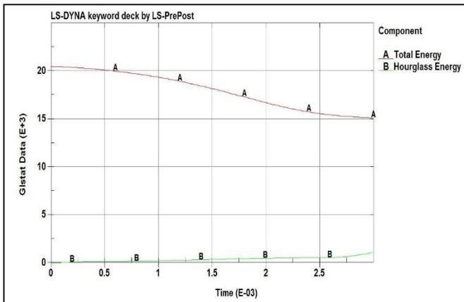
Fig 8: Total Energy and Hourglass Energy of A-Sandwich Panel.
