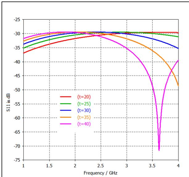
Fig 3: Core Thickness Study on EM Performance.
