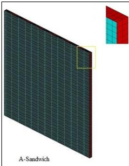
Fig 1: FE model of A-Sandwich Specimen.
