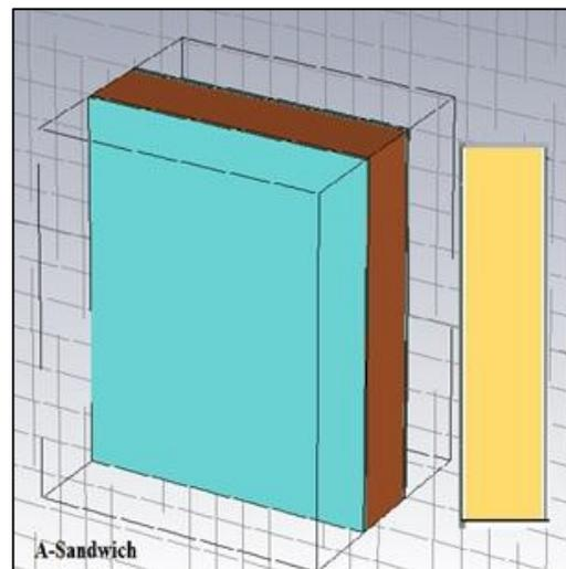
Fig 2: A-Sandwich Specimen subjected to EM Simulation.
