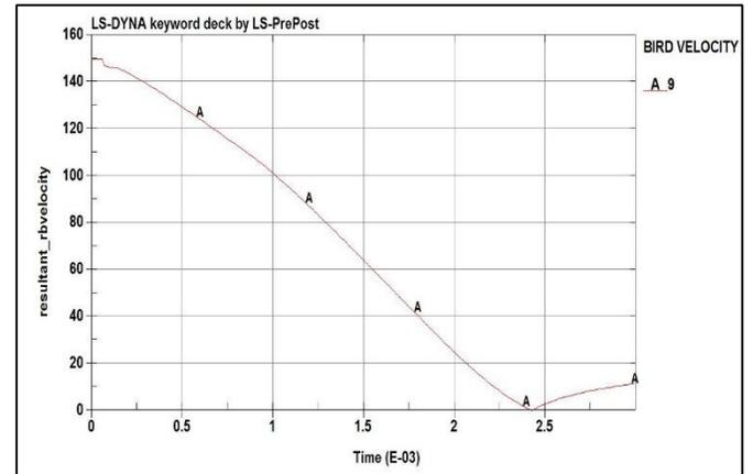
Fig 6: Bird velocity during impact of A-Sandwich Panel.
