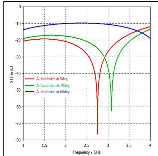
Fig 9: Return Losses of A-Sandwich panel at different angle of incidence.
