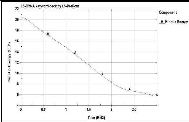
Fig 7: Kinetic Energy of the bird for A-Sandwich Panel.
