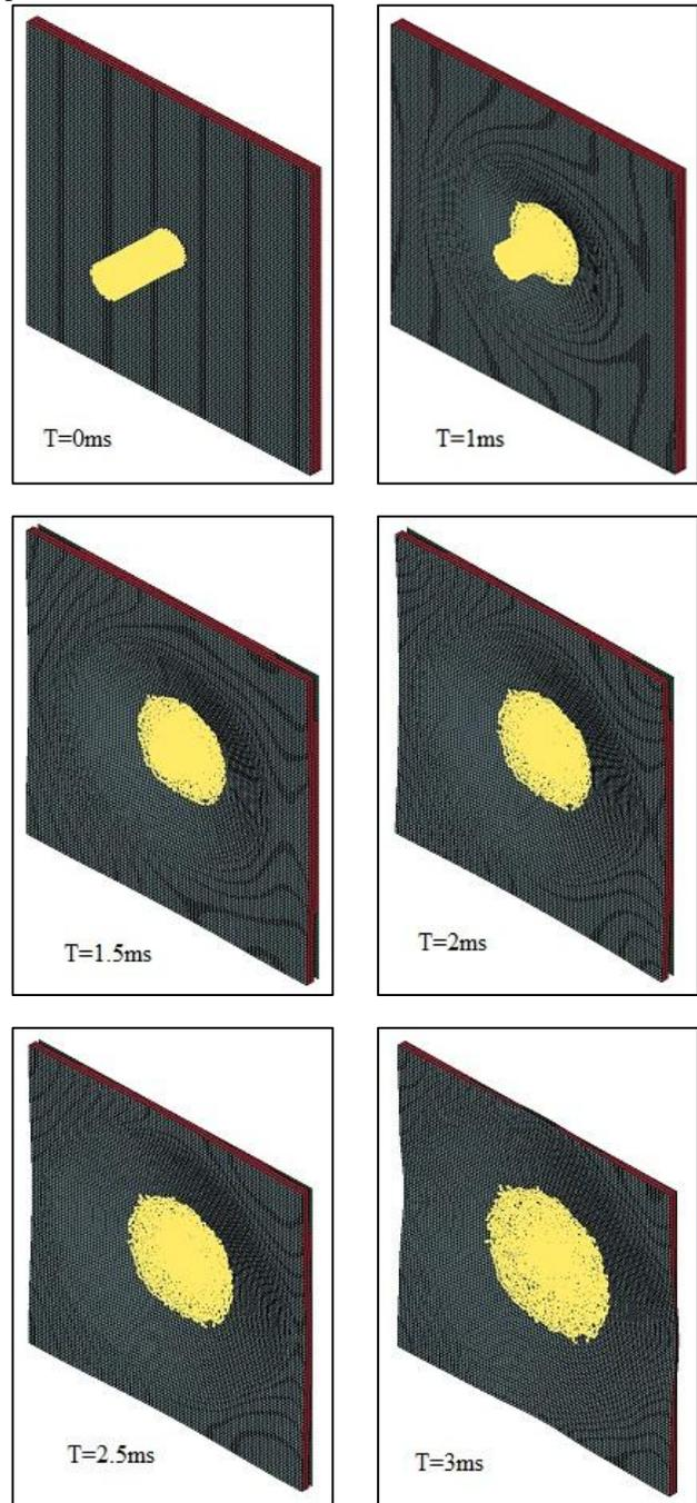
Fig 5: Bird Impact on A-Type Sandwich Specimen at different Time Intervals.
