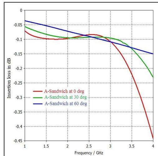
Fig 10: Insertion losses of A-Sandwich panel at different angle of incidence
