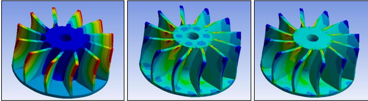
Fig 5: Deformation, Stress and Strain for Present Micro Gas Turbine (Titanium Alloy).
