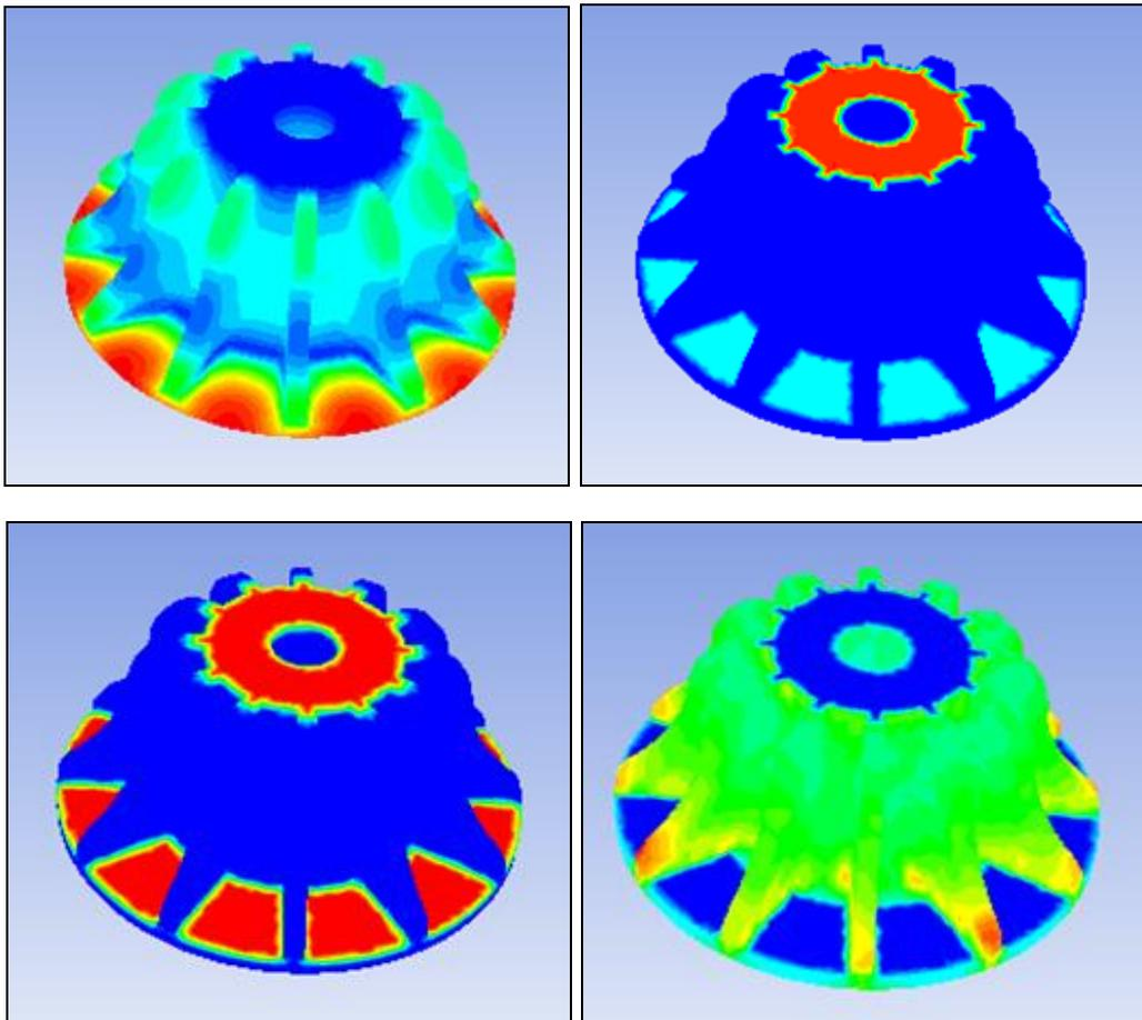
Fig 10: Pressure, Velocity, Temperature and HTC at  $V = 540$  m/s.
