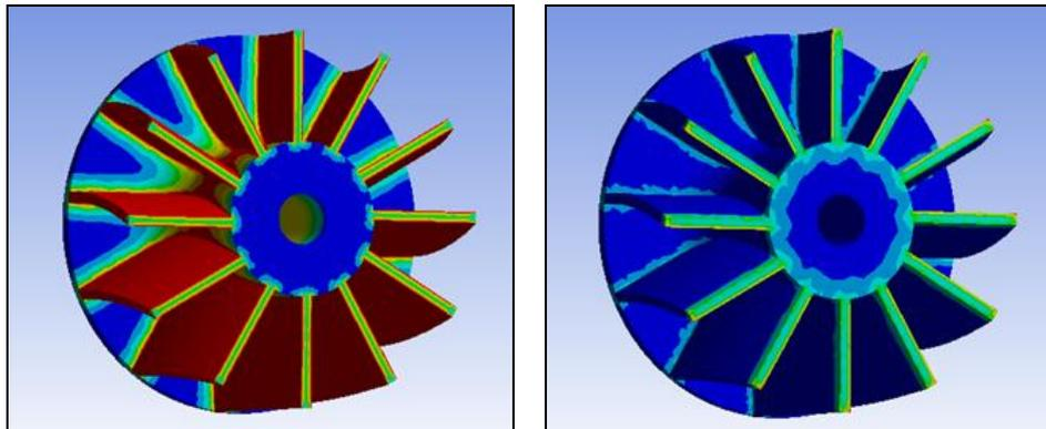
Fig 7: Temperature and Heat Flux for Present Micro Gas Turbine (Nickel Alloy).
