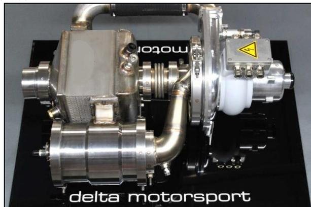
Fig 2: Micro Gas Turbine Used with Automobile Engine.
