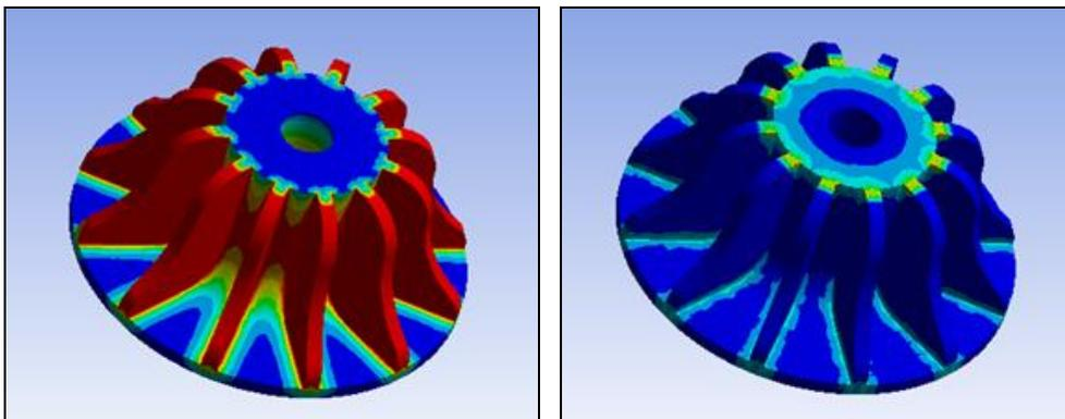
Fig 8: Temperature and Heat Flux for Modified Micro Gas Turbine (Nickel Alloy).
