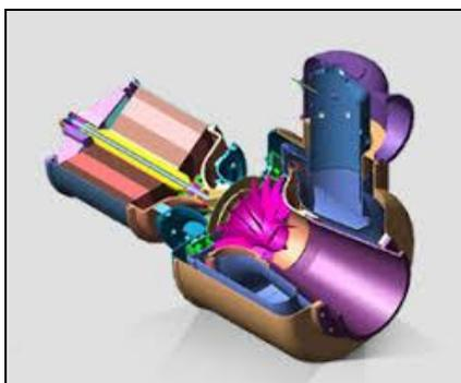
Fig 1: Micro Gas Turbine.
