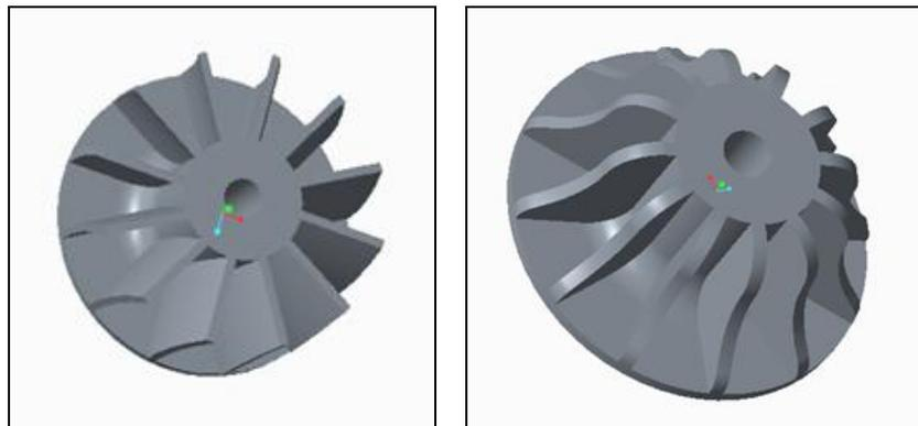
Fig 3: Present and Modified Micro Gas Turbine Model.
