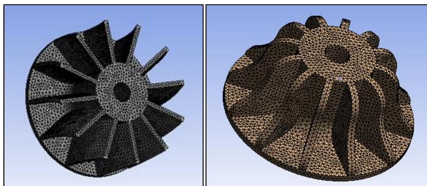
Fig 4: Present and Modified Mathematical Model of Micro Gas Turbine Model.
