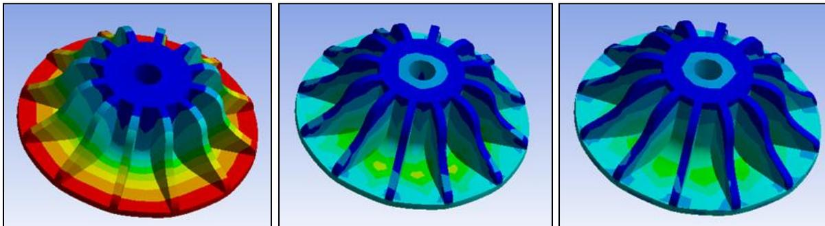
Fig 6: Deformation, Stress and Strain for Modified Micro Gas Turbine (Titanium Alloy).
