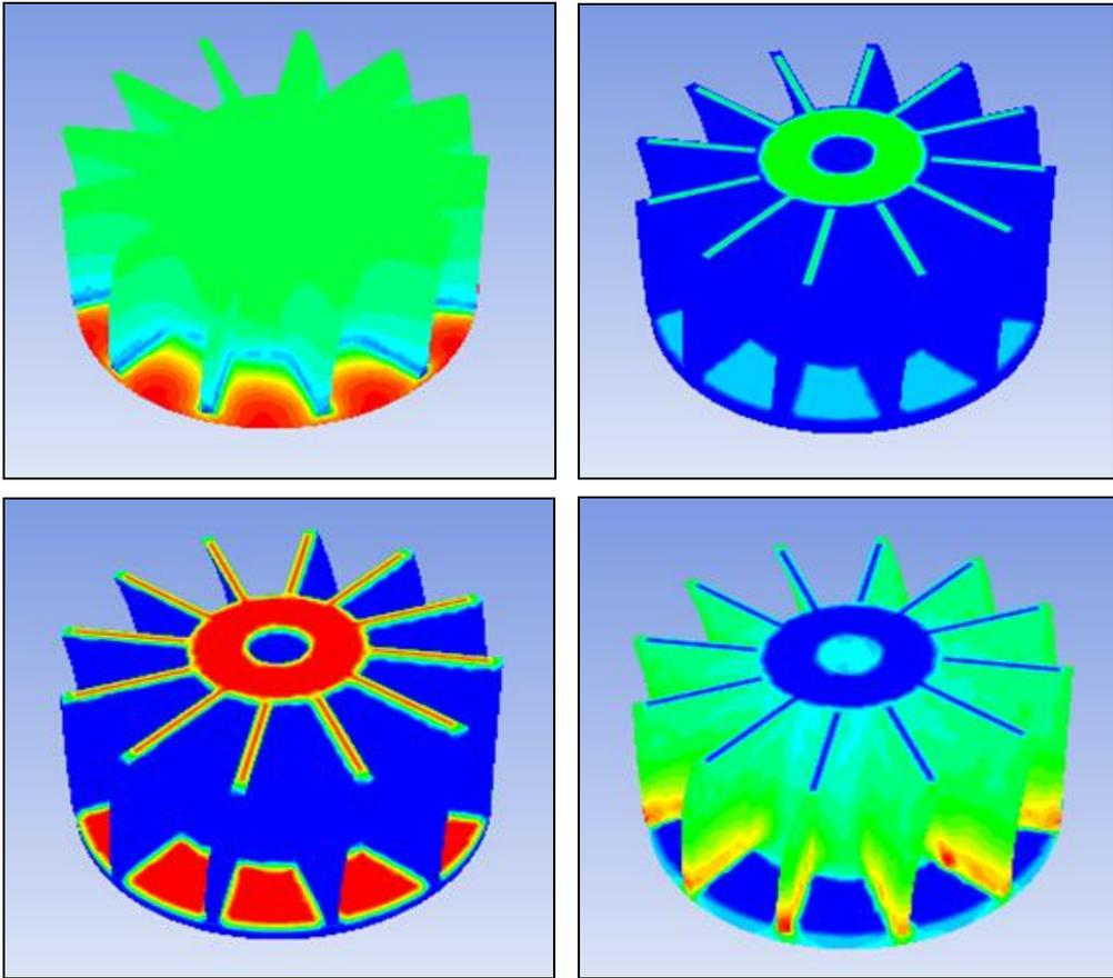
Fig 9: Pressure, Velocity, Temperature and HTC at  $V = 540$  m/s.
