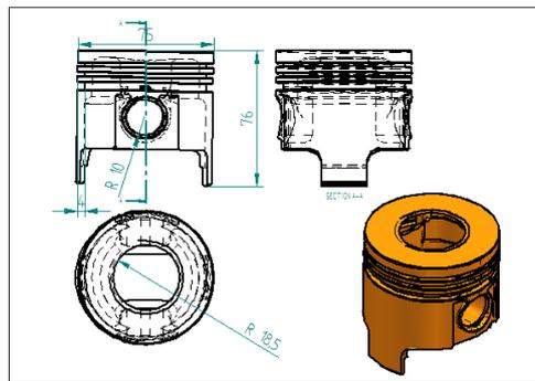
Fig1: Geometry of the Piston
