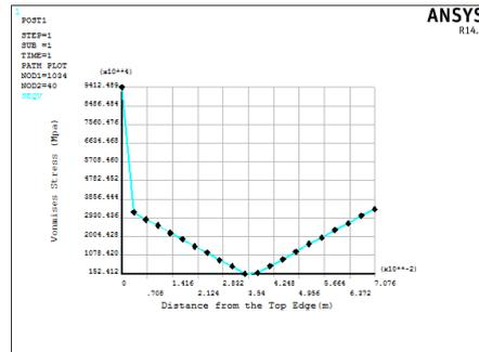
Fig8: Stress Variation with Thermal Barrier coatings
