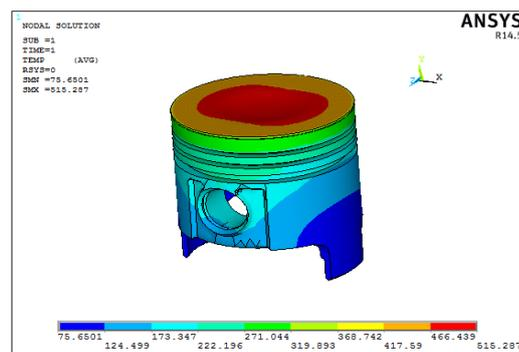
Fig10: Temperature Distribution with Thermal barrier Coatings
