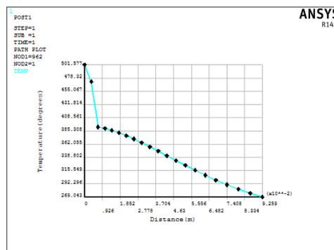
Fig6: Temperature Variaton with Thermal Barrier Coating
