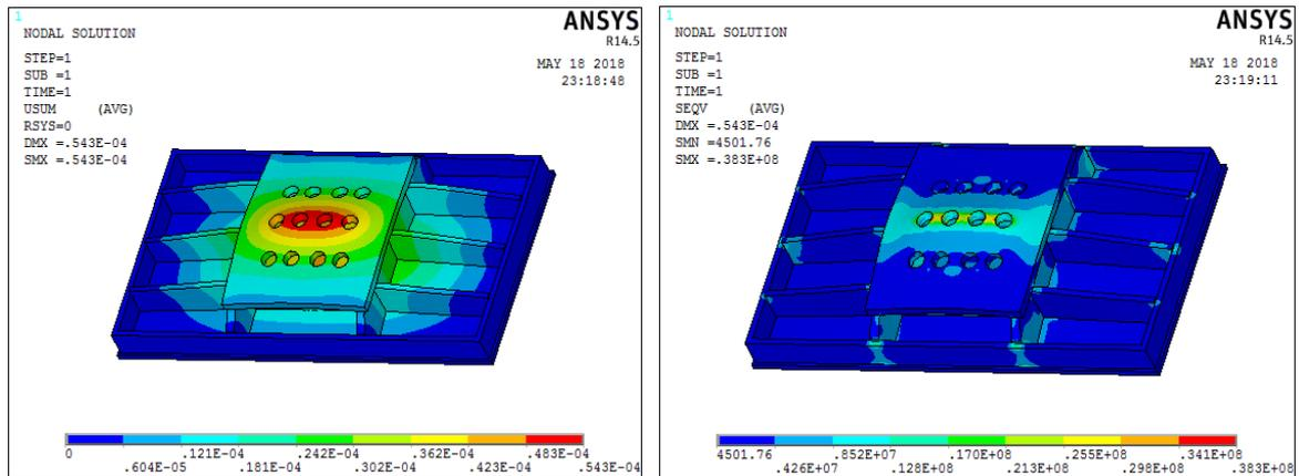
Fig 6: Displacement Plot for the Final Dimensions. Fig 7: Vonmises Stress in the Cylindrical Mount.
