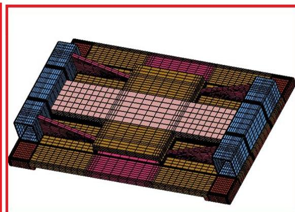
Fig3: Mesh of the Wall Bracket.
