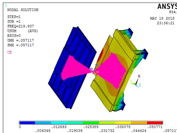
Fig 8: Mode Shape corresponding to the first fundamental Frequency.
