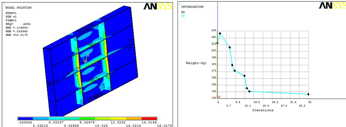
Fig 4: Vonmises Stress in the Final Set.
