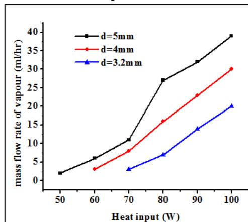
Fig 6: variation of vapor flow rate versus internal heat power for different tube diameters.
