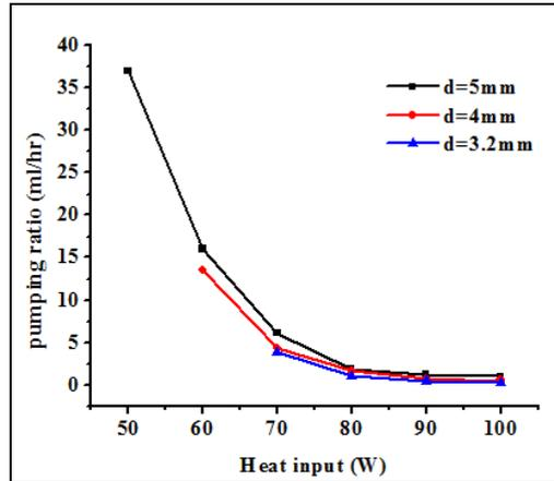
Fig 7: Variation of pumping ratio with heat input for different pump tube diameters.
