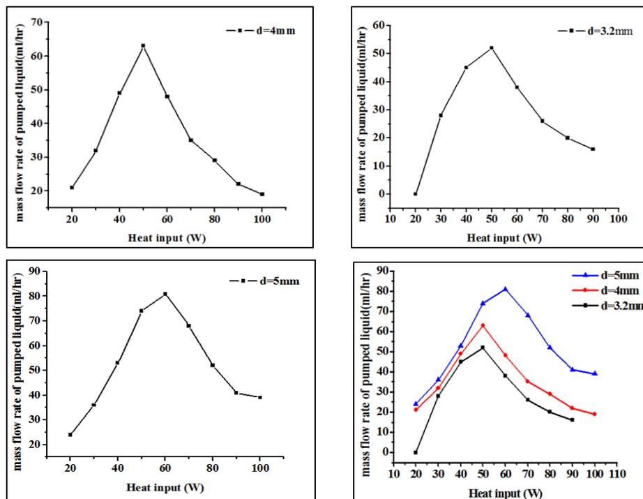
Fig 4 a, b, C & d: Variation of effect of pump tube diameters with mass flow rate of pumped liquid.
