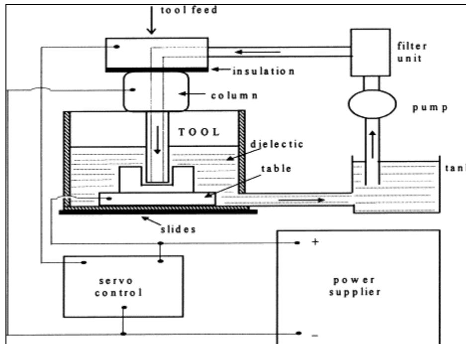
Fig 2: Schematic Representation of EDM Process.
