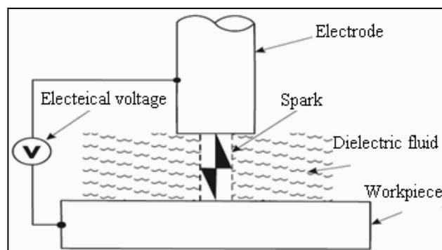
Fig 1: General Working Principal of EDM
