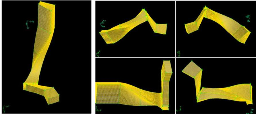
Fig 4: Meshed Centrifugal Impeller using Gambit
