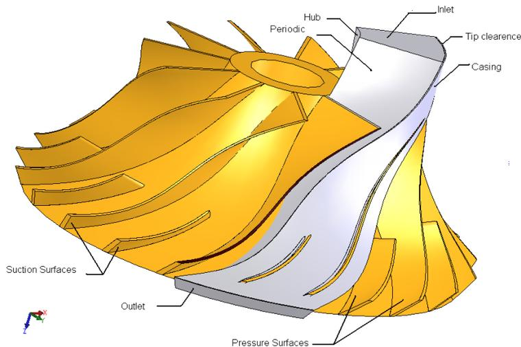
Fig 3: Centrifugal Impeller Model
