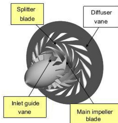
Fig1: Schematic of compressor
