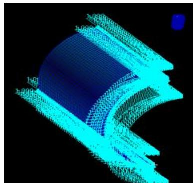
Fig 3: Meshing of Composite Drive Shaft. Fig 4: Boundary Conditions on the Composite Drive Shaft.
