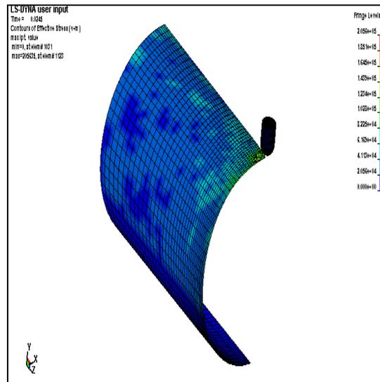
Fig 5: Stress Plots for HS Carbon/Epoxy Shaft with Lay-Up Configuration.
