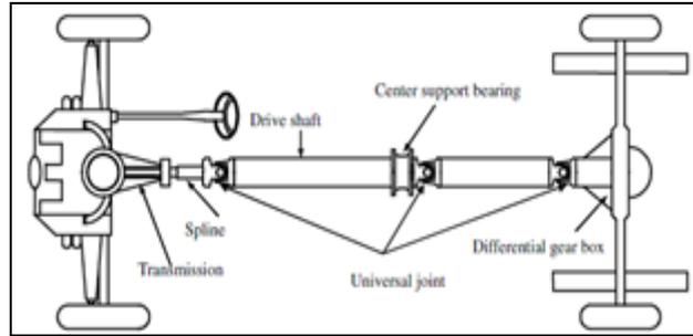
Fig 1: Conventional Two-Piece Steel Driveshaft [5].
