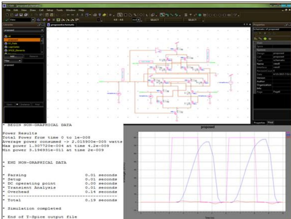
Fig 1: Schematic with simulation result of Double-Tail Comparator.
