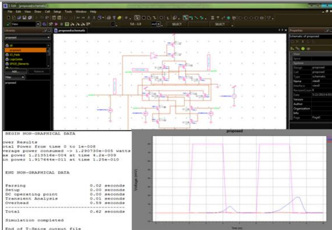
Fig 3: Schematic with simulation result of Proposed Double-Tail Comparator with Stack Technique.
