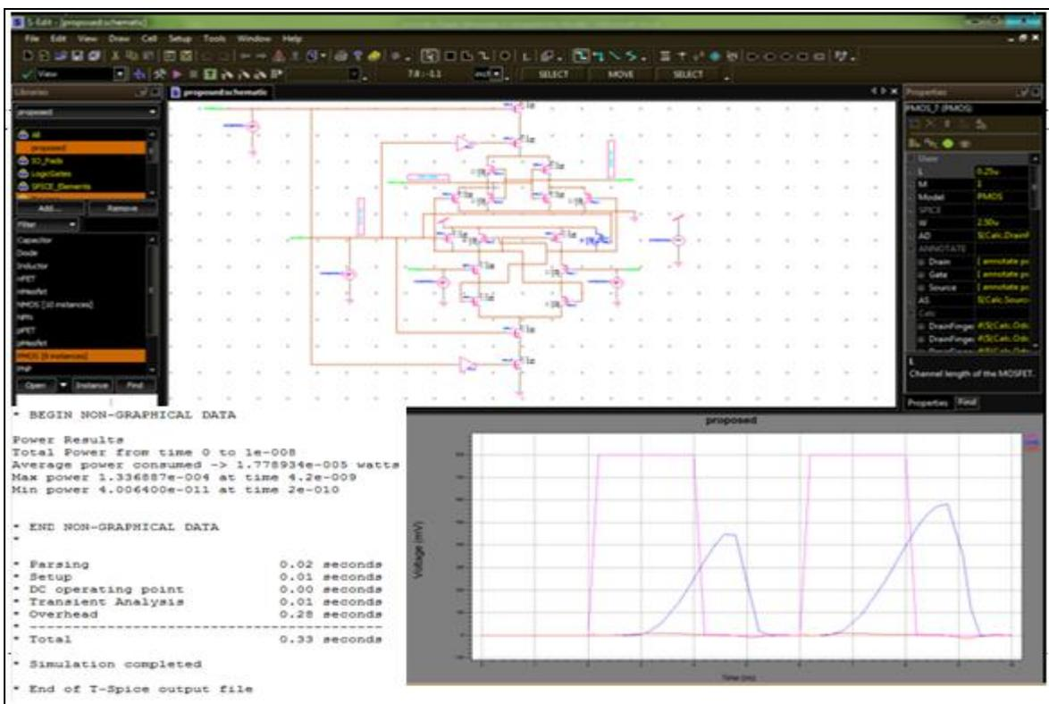
Fig 2: Schematic with simulation result of Proposed Double-Tail Comparator with Sleep Transistor Technique.
