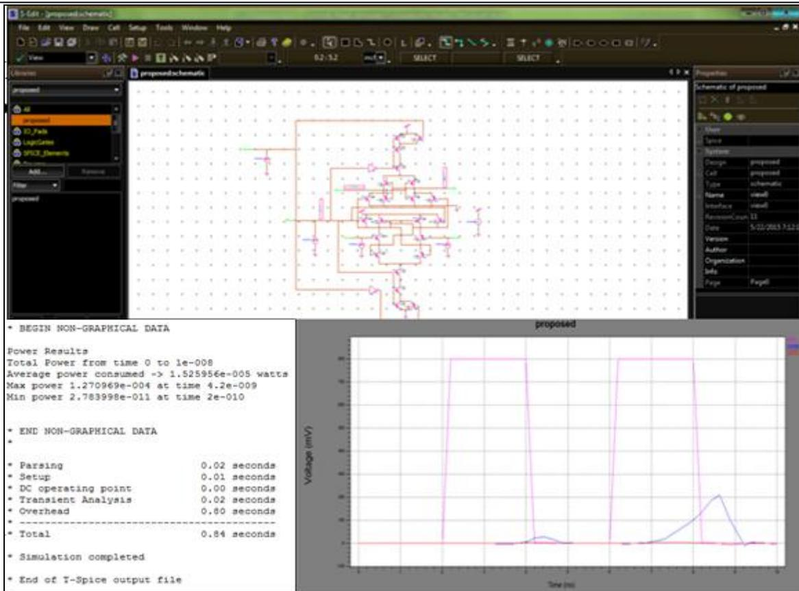
Fig 4: Schematic with simulation result of Proposed Double-Tail Comparator with Stack Technique.
