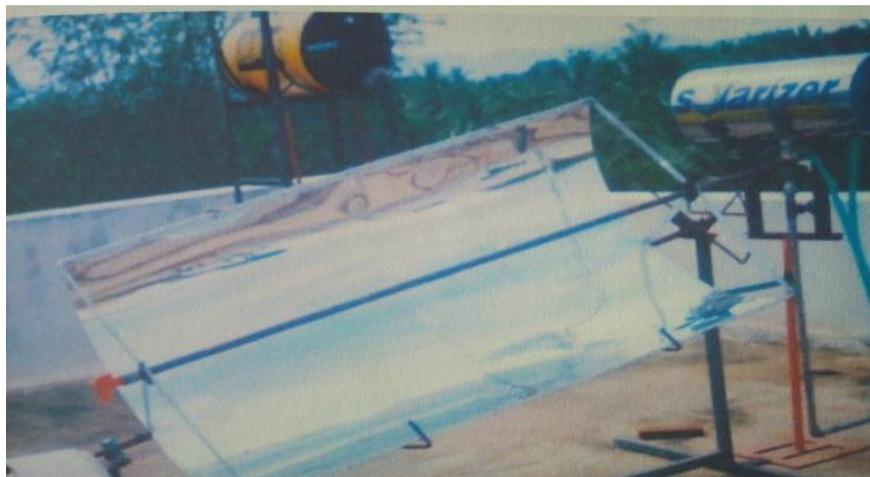
Fig 2: CPC with tracking system at SJCIT
