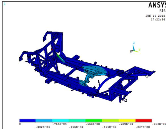
Fig 16: Displacement Plot (Lateral Spectrum)
