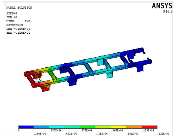
Fig 12: Displacement Plot (Longitudinal Spectrum)
