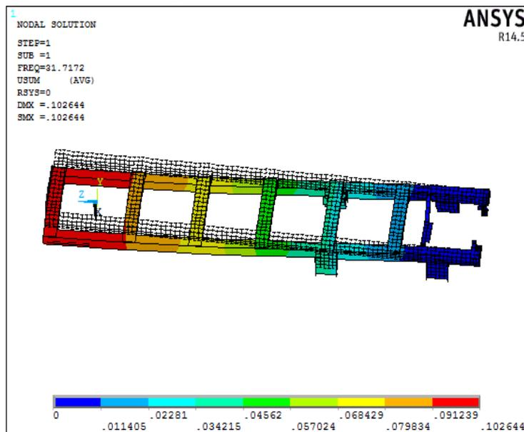
Fig 7: Mode Shape with un-deformed model.
