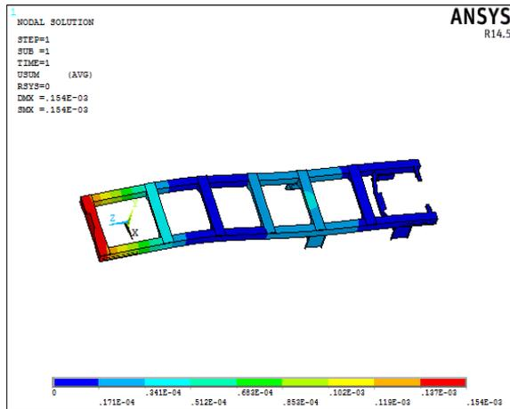
Fig 5: Displacement for Self Weight.
