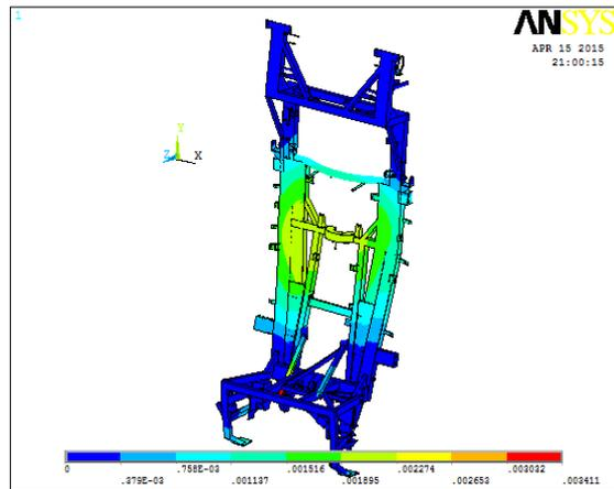
Fig 9: Displacement for External Load.
