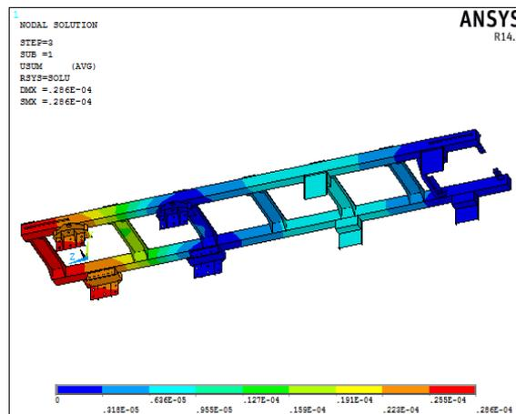
Fig 15: Displacement Plot (Lateral Spectrum)
