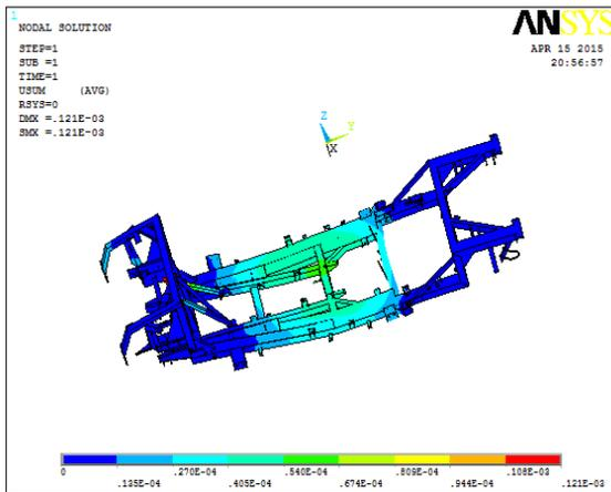
Fig 8: Displacement for Self Weight.
