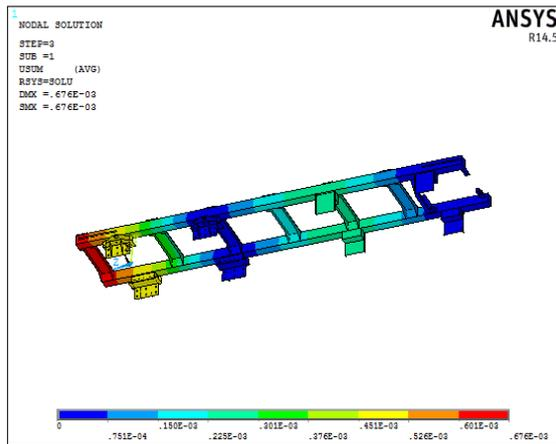
Fig 11: Displacement Plot (Vertical Spectrum)
