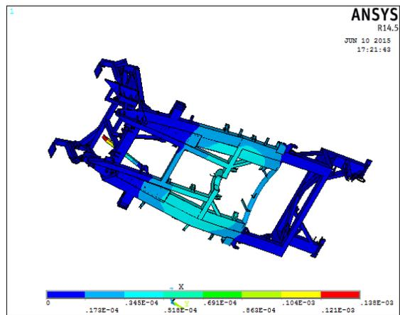
Fig 14: Displacement Plot (Longitudinal Spectrum)
