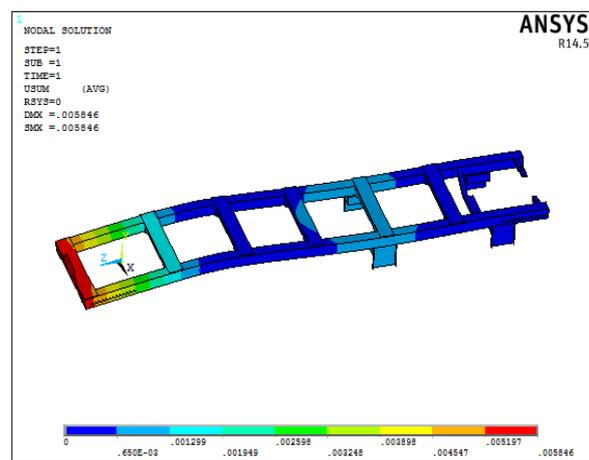
Fig 6: Displacement for External Load.
