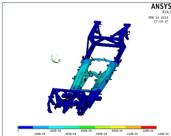
Fig 13: Displacement Plot (Vertical Spectrum)
