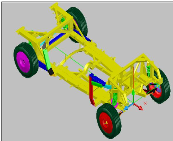
Fig 3: Simulation view of Chassis
