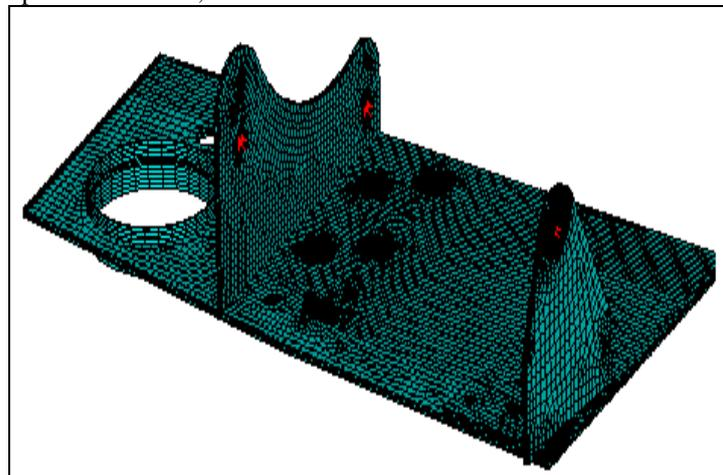
Fig 1: Meshing of Control Unit Bracket.
