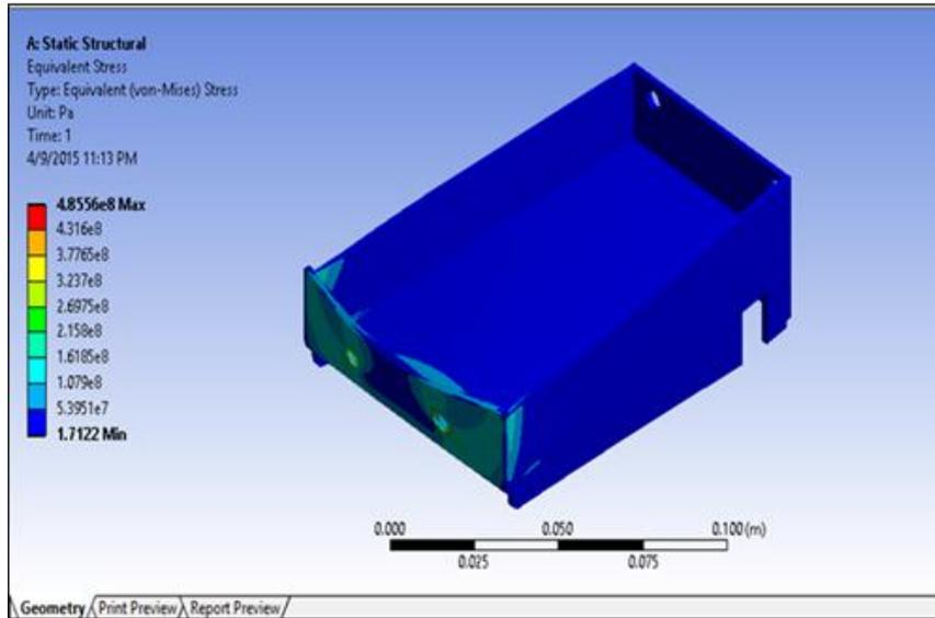
Fig 5: Contour Plot of the Equivalent von-Misses Stresses Acting on the Member.
