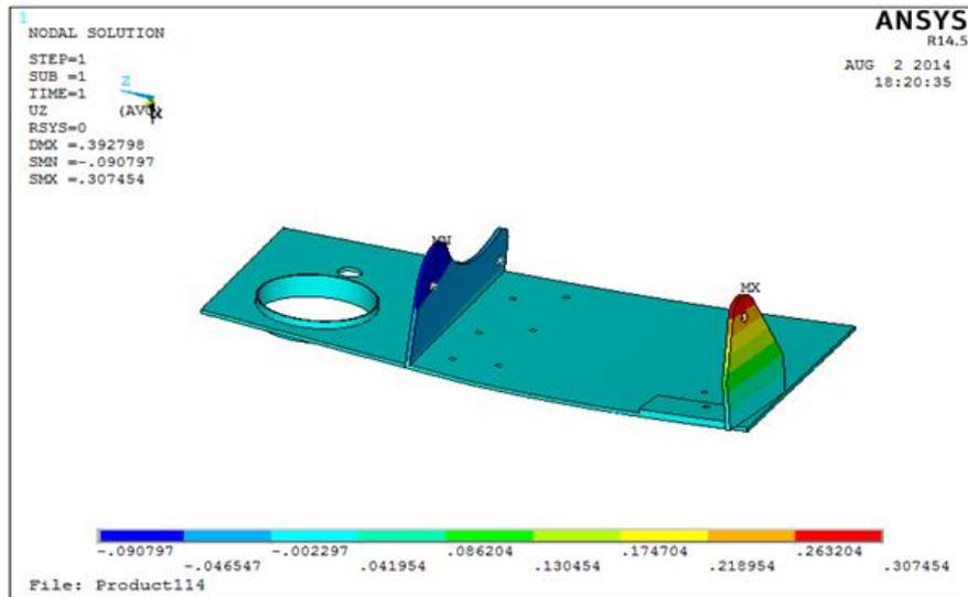
Fig 6: Contour Plot of Displacement along Z Direction.
