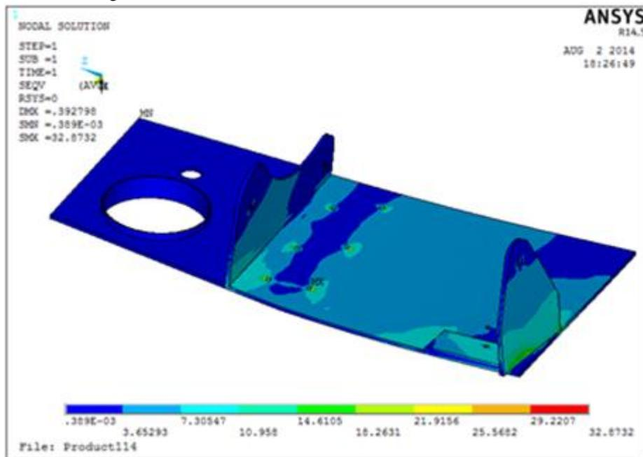
Fig 4: Contour Plot of the Tri-Axial Principal Stresses Acting on the Member.
