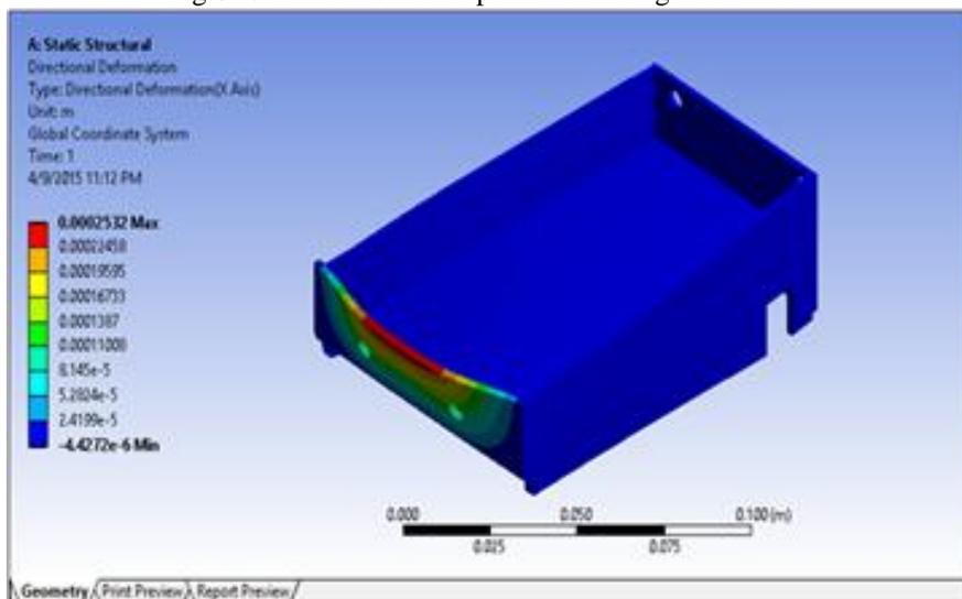
Fig 7: Contour plot of Directional Deformation along X Axis.
