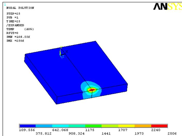
Fig 2: Temperature at Start, Middle and End due to Welding Process.
