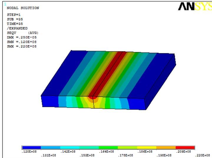
Fig 4: Structural Results for given Heat flux of  $4e7w/m^2$ .
