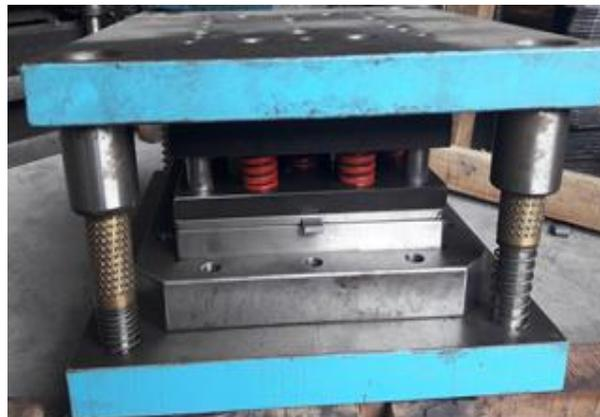
Fig 7: Progressive Press Tool for Stage 01.
