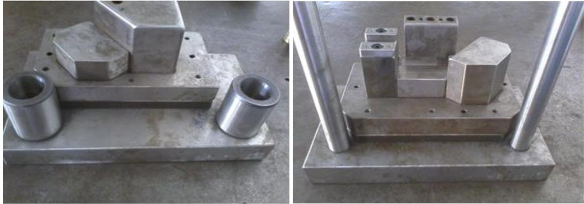
Fig 8: Forming Press Tool for Stage 02.
