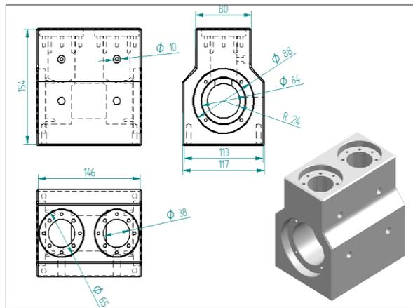
Fig 7: Cam Box Assembly.
