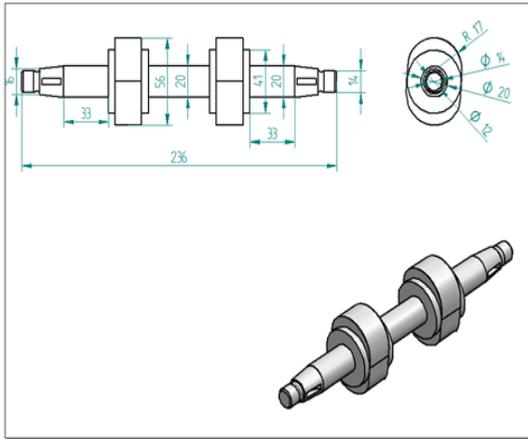
Fig 6: Cam Shaft Dimensions (mm).
