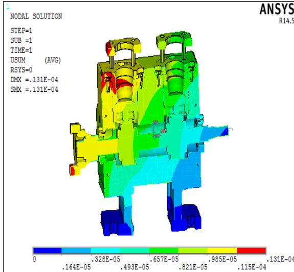
Fig 13: Displacement Plot.
