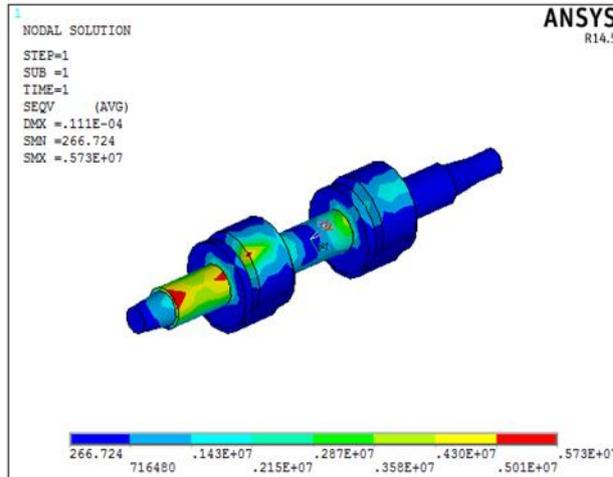
Fig 15: von-Mises Stress Developed in the Cam Shaft.
