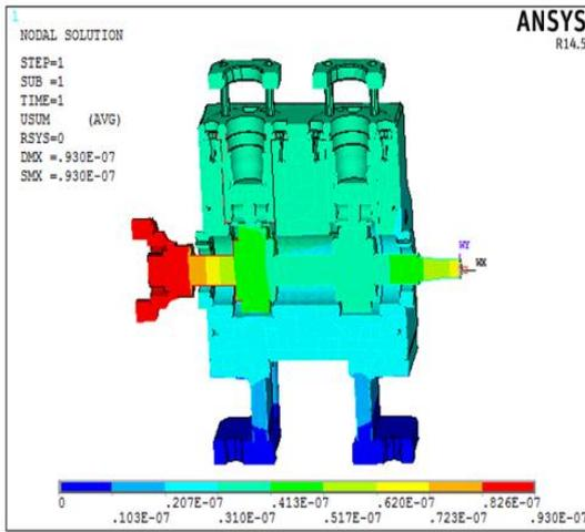
Fig 11: Displacement Plot.
