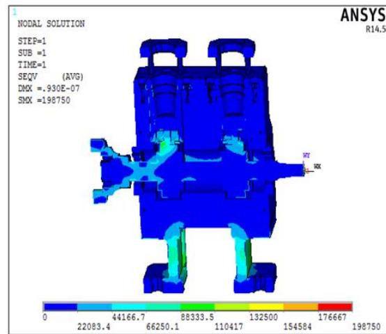
Fig 12: von-Mises Stress Plot.
