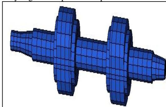
Fig 9: Brick Mesh of the Shaft Structure.
