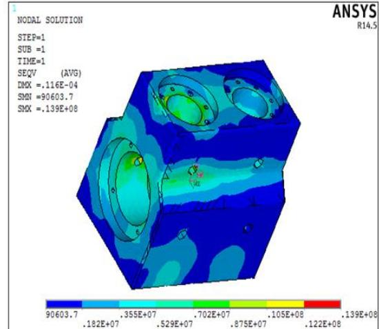
Fig 16: von-Mises Stress in the Cam Box.
