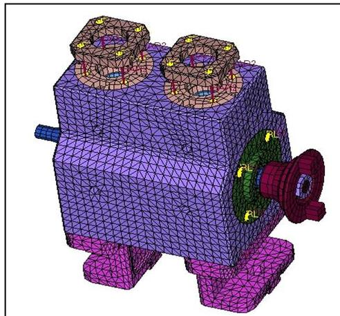
Fig 8: Mesh view of the Cam Box Assembly.
