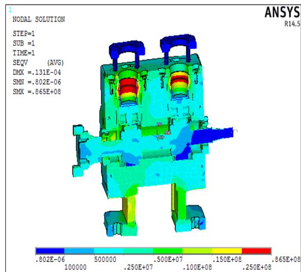
Fig 14: von-Mises Stress Development due to External Loads.
