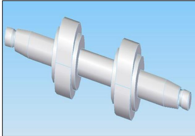
Fig 4: Two Lobe Cam Shaft.
