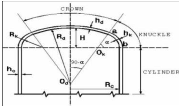
Fig 2: Dome Resembling Torispherical Heads of Pressure Vessel.
