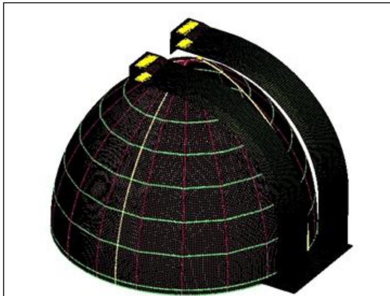
Fig 3: Finite Element Representation of the Dome Structure.
