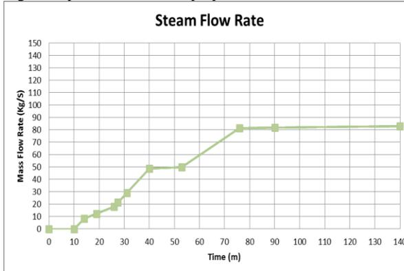
Fig 13: Upstream steam flow rate of a hot start. Table 2: HTC at Different Zones.
