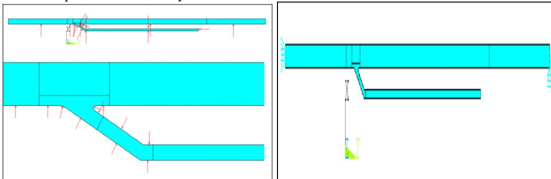
Fig 16: Steam Pressure and Boundary Constraints.
