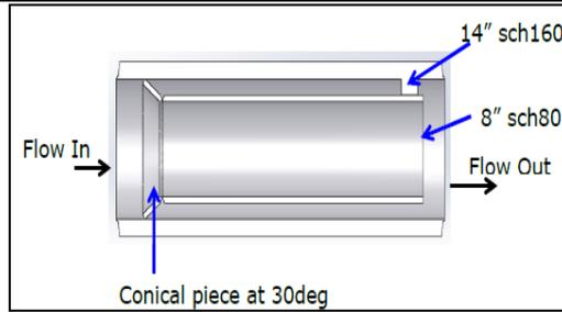
Fig 4: Sectional View (before weld).
