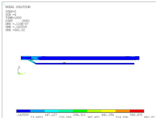
Fig 19: Stress intensity (SINT) contour at 1800sec.
