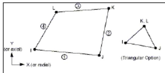
Fig 8: PLANE55 Geometry.
