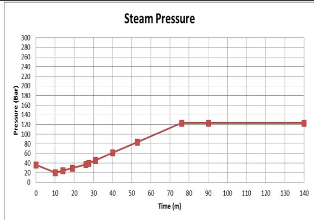
Fig 12: Upstream steam pressure operation of a hot start.
