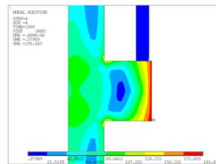
Fig 25: Maximum Stress at stopper.
