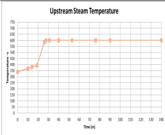
Fig 11: Upstream steam temp operation of a hot start.
