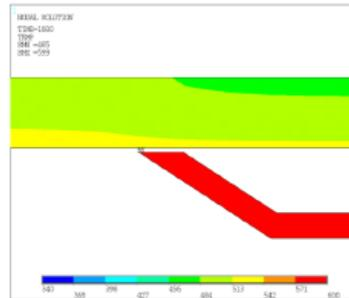
It can be observed that full main steam pipe is getting heated up in a synchronous manner. Liner & liner supports are also getting heated up.
