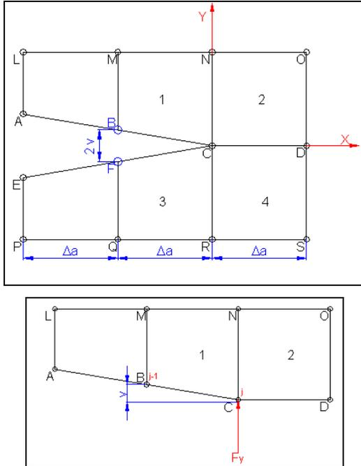
Fig 1: MVCCI Model Showing Displacement Adjacent to Crack Tip and Reaction Force at Crack Tip.
