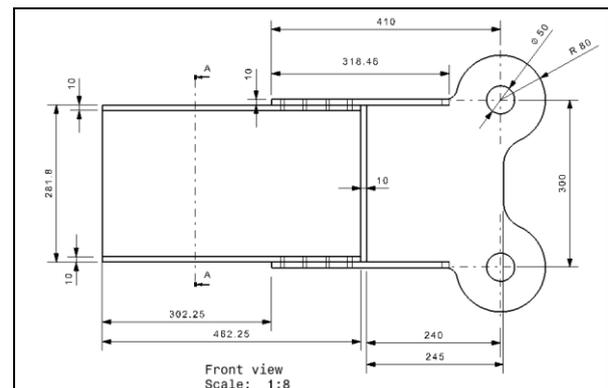
Fig 2: Front View of Assembly.
