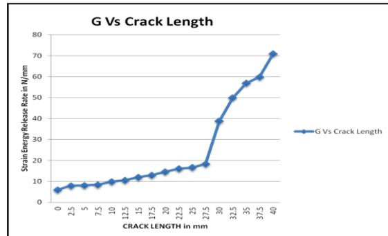
Fig 9: 'G' versus Crack length.
