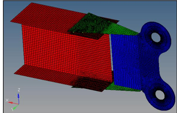
Fig 5: 2D FE Model of the Wing Fuselage Attachment Bracket.
