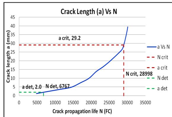
Fig 11: 'a' Vs Crack Propagation Life.
