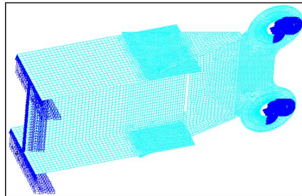
Fig 6: Loads and Boundary Conditions.
