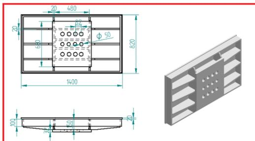
Fig4 : Three dimensional Geometry of the Cylinder Mount
