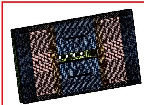
Fig5 : Mesh of the Cylinder Mount
