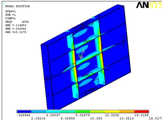
Fig8; Vonmises Stress Plot in the Ribbed Configuration
