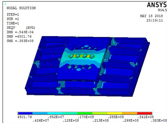
Fig9: Vonmises Stress in the cylinder mount
