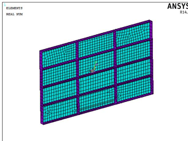
Fig3 : Mesh Plot of the Simplified Geometry
