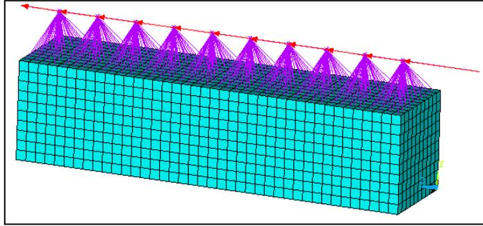
Fig 3: Snap shot of finite element model highlighting the direction of flow (red colored arrows)
