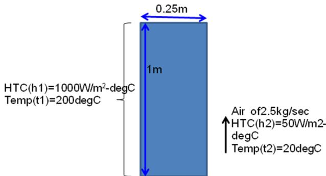
Fig 5: Boundary conditions of the block
