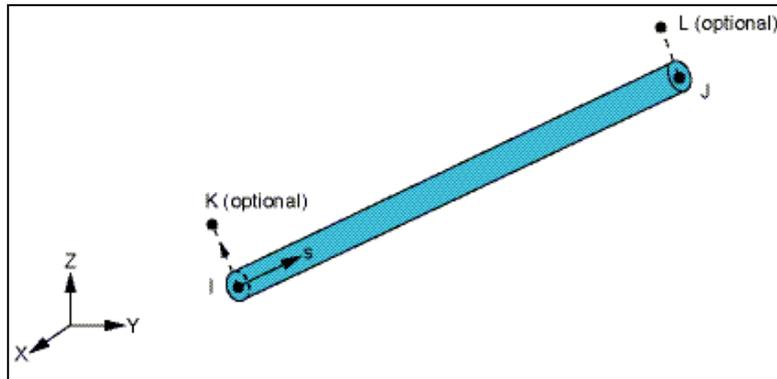
Fig 1: Element topology of Fluid116
