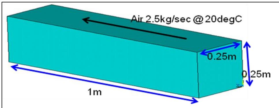
Fig 2: A block of 1mX0.25mX0.25m
