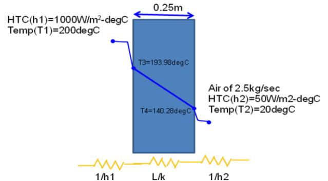
Fig 6: Analytical model highlighting heat resistance
