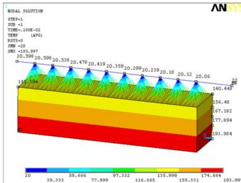
Fig 7: Steady state temperature contour with heated source at bottom face (in degC)
