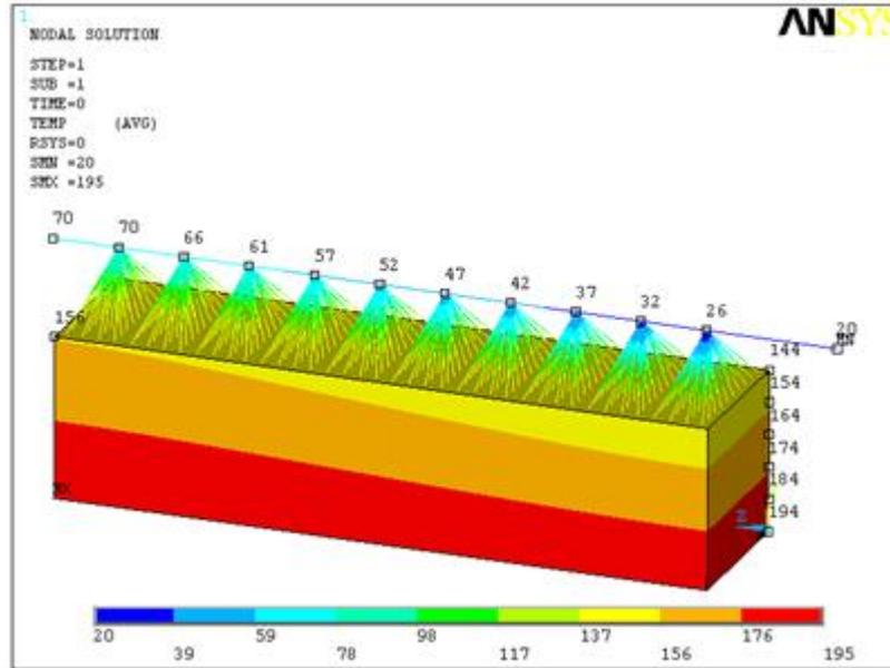
Fig 8: Steady state temperature contour with reduced air flowrate (in degC)
