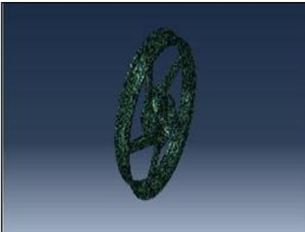
Fig 3: Meshed model of 5 spoke alloy wheel
