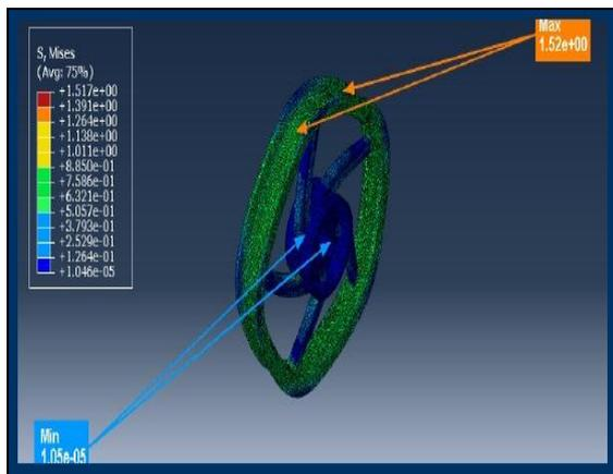
Fig 8: von-Mises stress distribution plot
