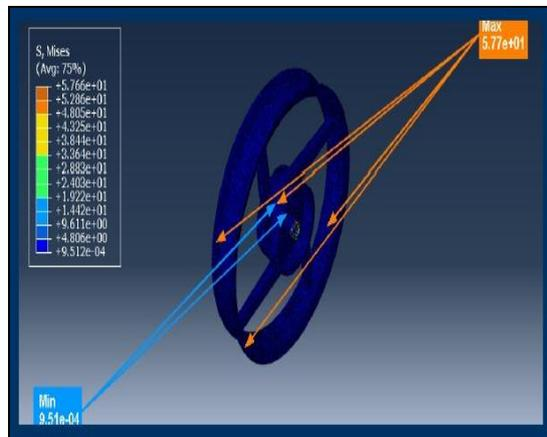
Fig 12: Von-Mises distribution stress plot
