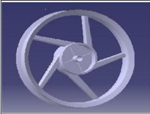
Fig 1: 3D model of 5 spoked alloy wheel
