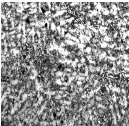
Fig 8: Microstructure of Nihard4 steel before treatment
