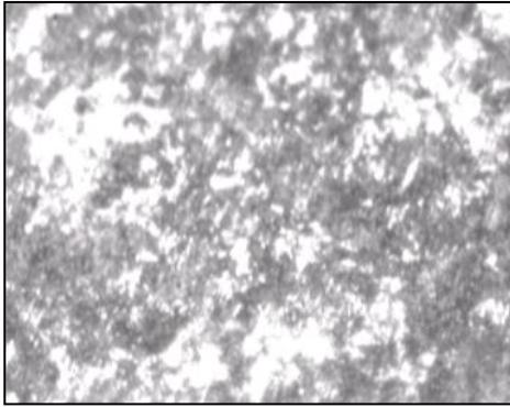
Fig 4: Microstructure of spring steel before treatment
