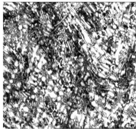
Fig 9: Microstructure of Nihard4 steel after treatment
