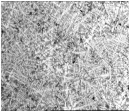
Fig 6: Microstructure of High Chromium steel before treatment
