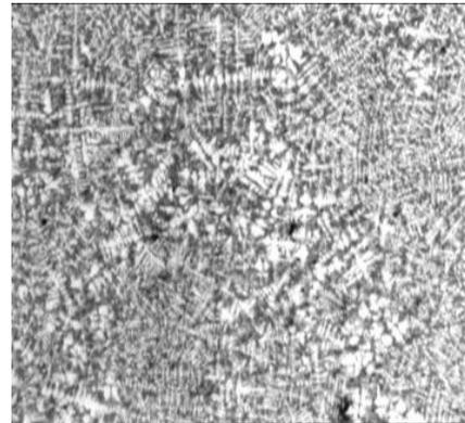
Fig 7: Microstructure of High Chromium steel after treatment
