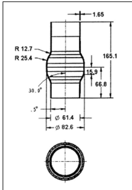
Fig 1: Part geometry formed in the experiment is a tube with axisymmetric bulge
