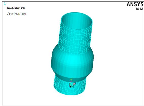
Fig 3: Geometry of Meshed Model
