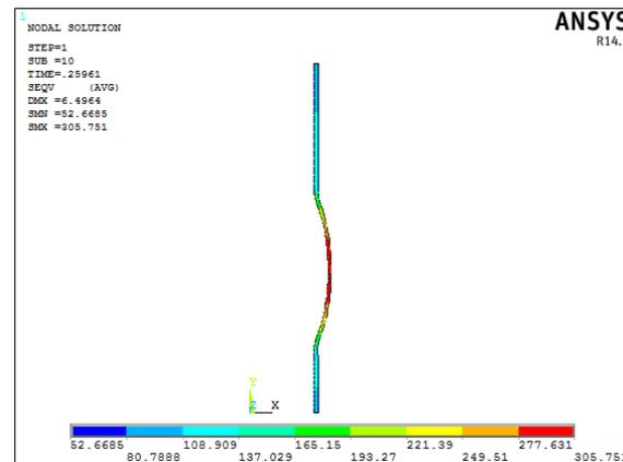
Fig 7: von Mises stress at time = 0.25961seconds
