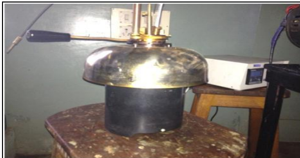
Fig 4.2: Pensky–Martens closed cup test
