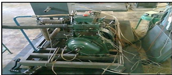
Fig 5.1(a): Photographic view of TV1, Kirloskar made, 4 Stroke Single Cylinder Engine.
