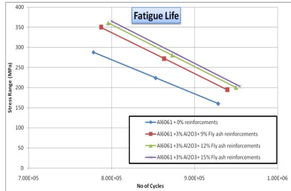
Fig 6: S-N curve for unreinforced alloy and Hybrid Composite material.
