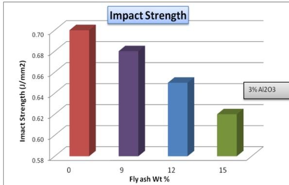
Fig 5: Impact strength vs Fly Ash wt %
