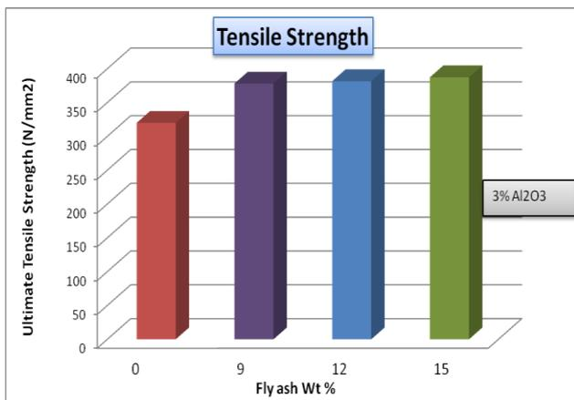
Fig 3: Tensile Strength vs Fly Ash wt %
