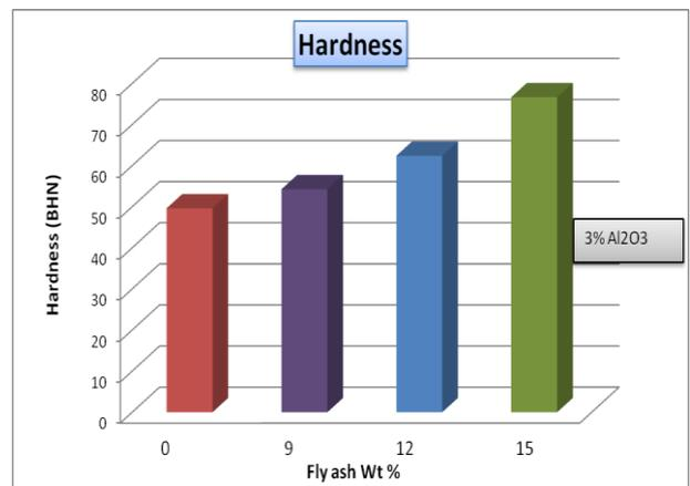
Fig 4: Hardness vs Fly Ash wt %
