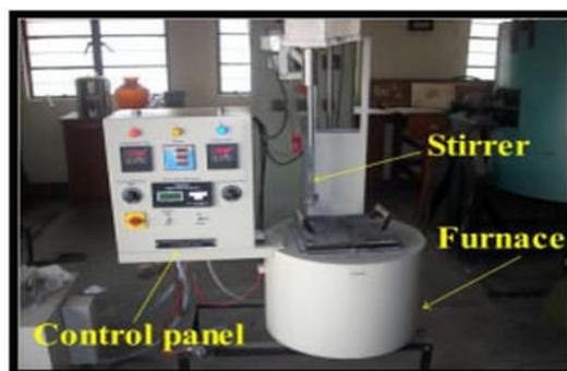
Fig 1: Stir Casting Set up
