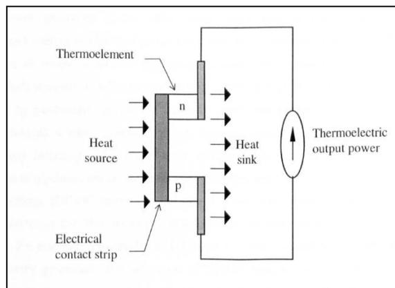
Fig 1.3: Working of thermoelectric devices.
