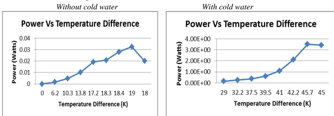
Fig 5.2: Power output as a function of temperature difference.
