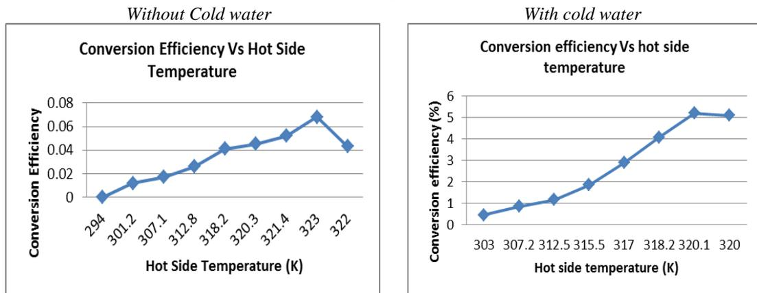
Fig 5.4: Conversion efficiency Vs hot side temperature
