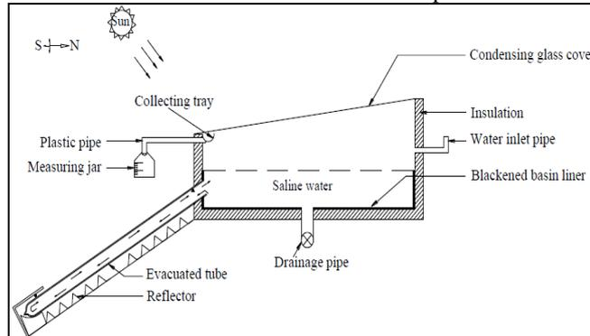
Fig 1.4: Schematic diagram of Single Basin Solar Still with evacuated tubes.
