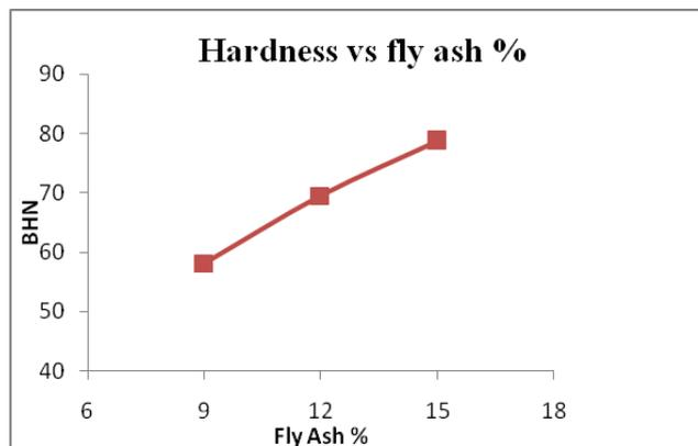
Fig 4.3: BHN V/S fly ash Weight %.
