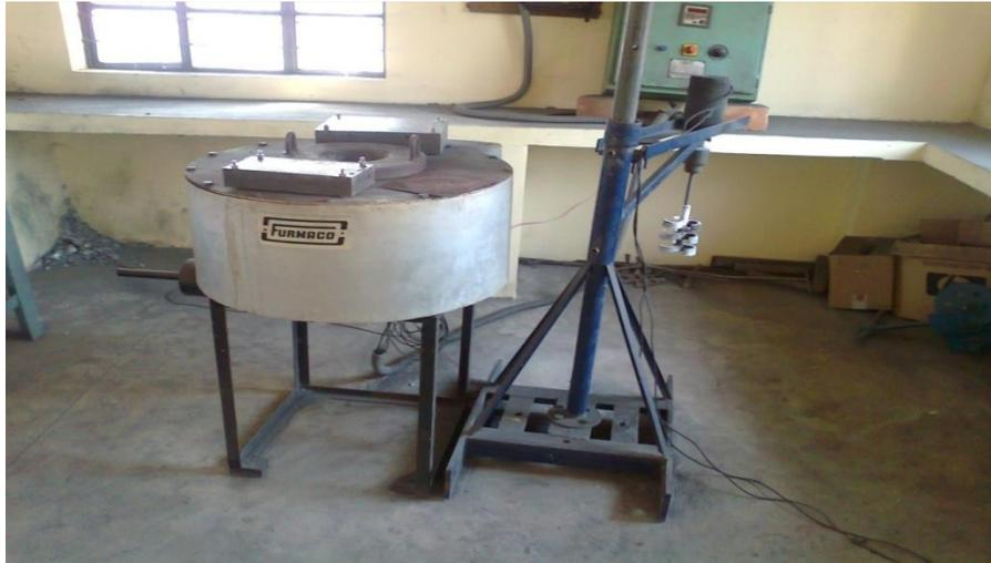
Fig 3.1: Stir casting.
