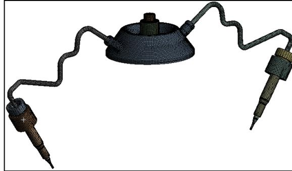
Fig 2.1: Meshed Model of the EGT Sensor.
