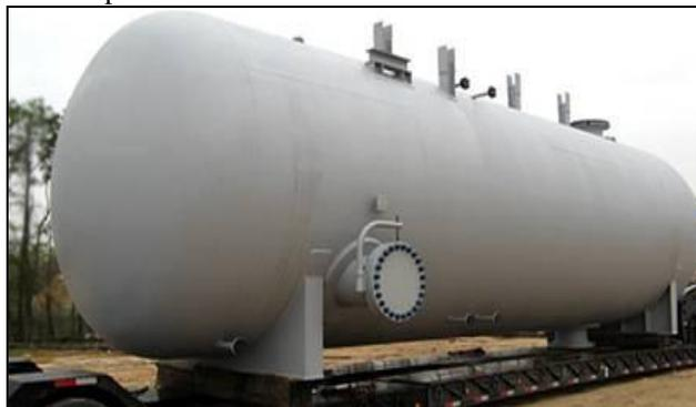
Fig 1: Pressure Vessel.
