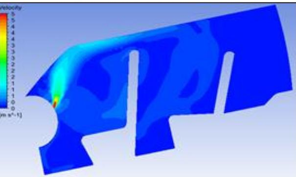
Fig 13: Temperature and Velocity Contours at Rating Plane 3 for Iteration 2.
