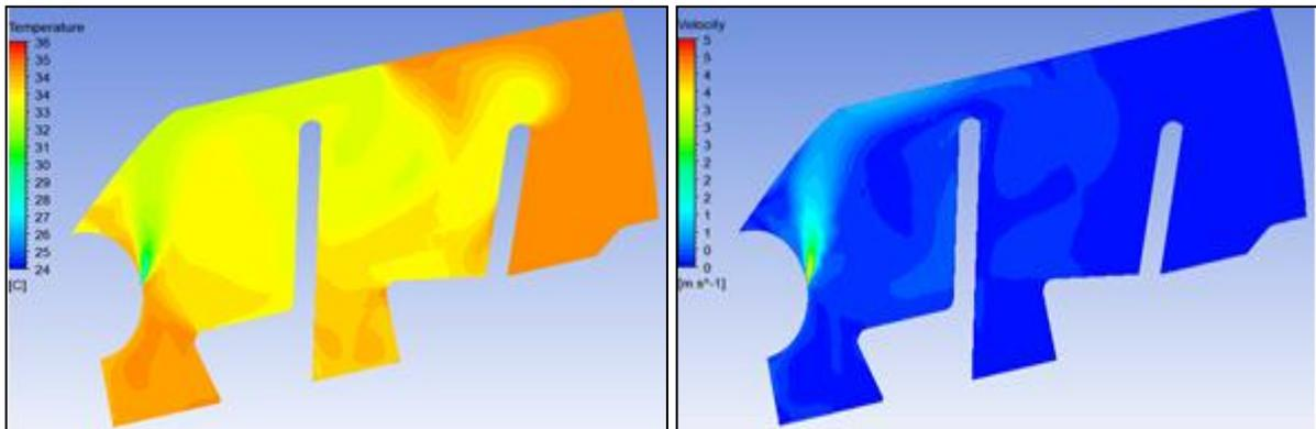
Fig 6: Temperature & Velocity Contours at Rating Plane 2 for Iteration 1.
