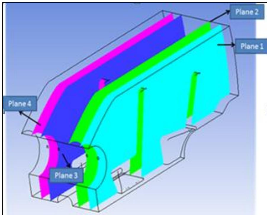
Fig 4: Post-Processing: Rating Planes at each Vent Location.
