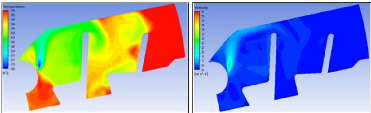
Fig 8: Temperature & Velocity Contours at Rating Plane 4 for Iteration 1.
