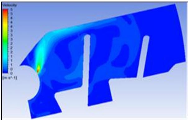
Fig 12: Temperature and Velocity Contours at Rating Plane 2 for Iteration 2.
