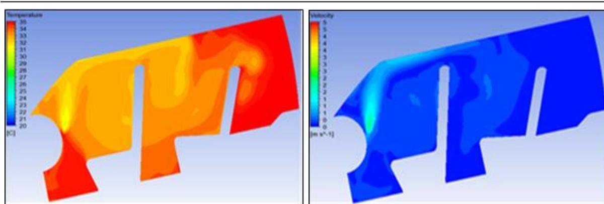
Fig 14: Temperature and Velocity Contours at Rating Plane 4 for Iteration 2.
