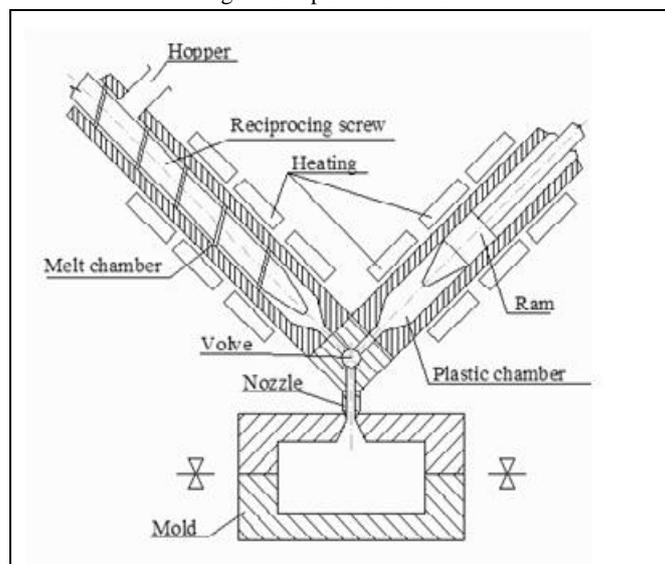
Fig 3: Schematic of rep rt9 Vertical Injection Mould Machine.
