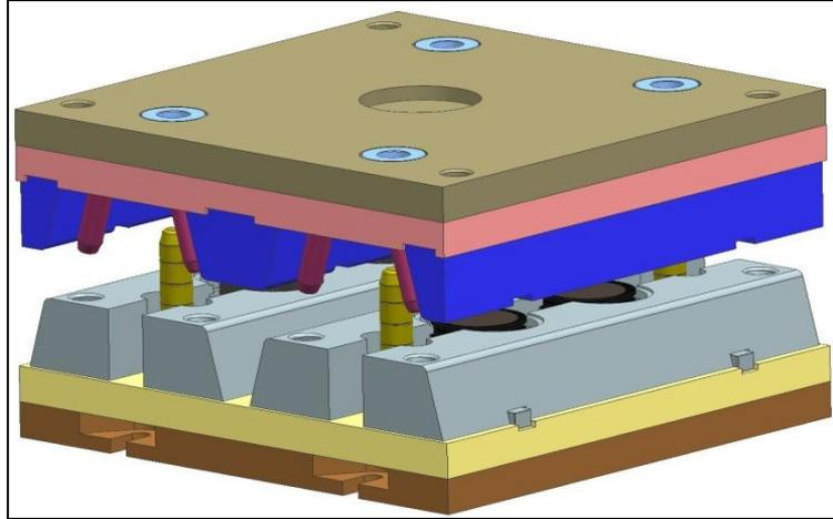
Fig 13: Mould Opening With Finger Cam Actuation Method.
