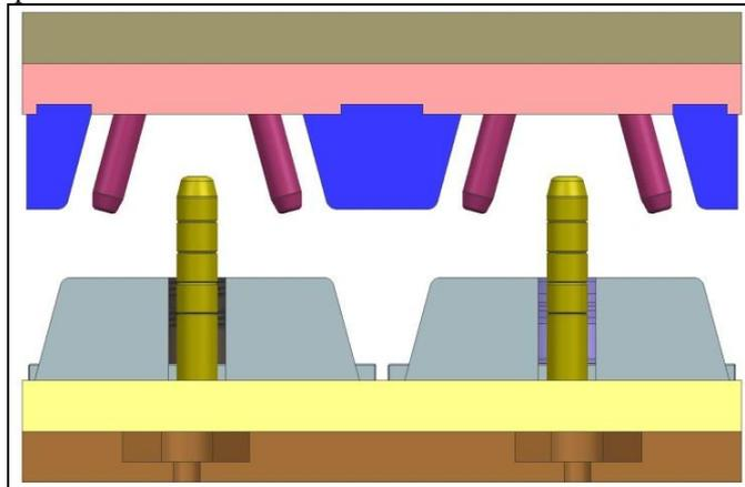
Fig 7: 3D Model of Our Injection Mould with Finger Cam Actuation Method.
