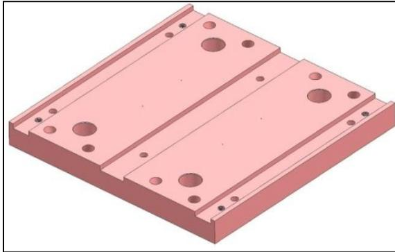
Fig 8: Cavity Plate.
