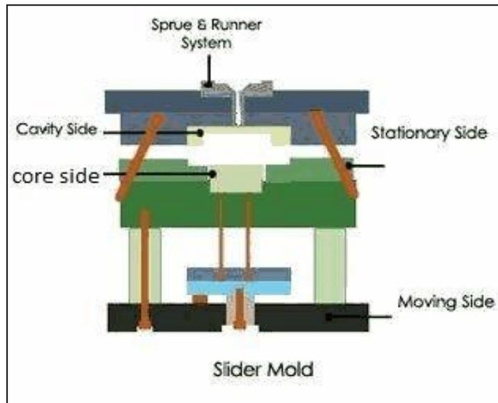
Fig 6: Standard Two Plate Mould (Concept-3).
