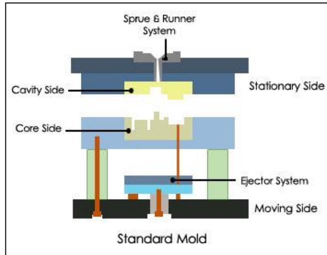
Fig 4: Standard Two Plate Mould (Concept-1).
