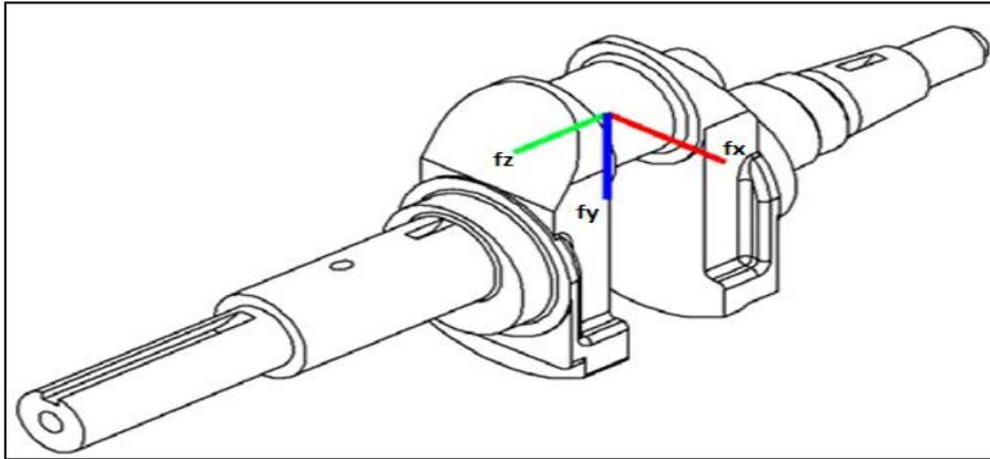
Fig 4: Boundary Condition for the Crankshaft Model.
