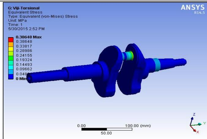
Fig 7: Effect of Torsional Load
