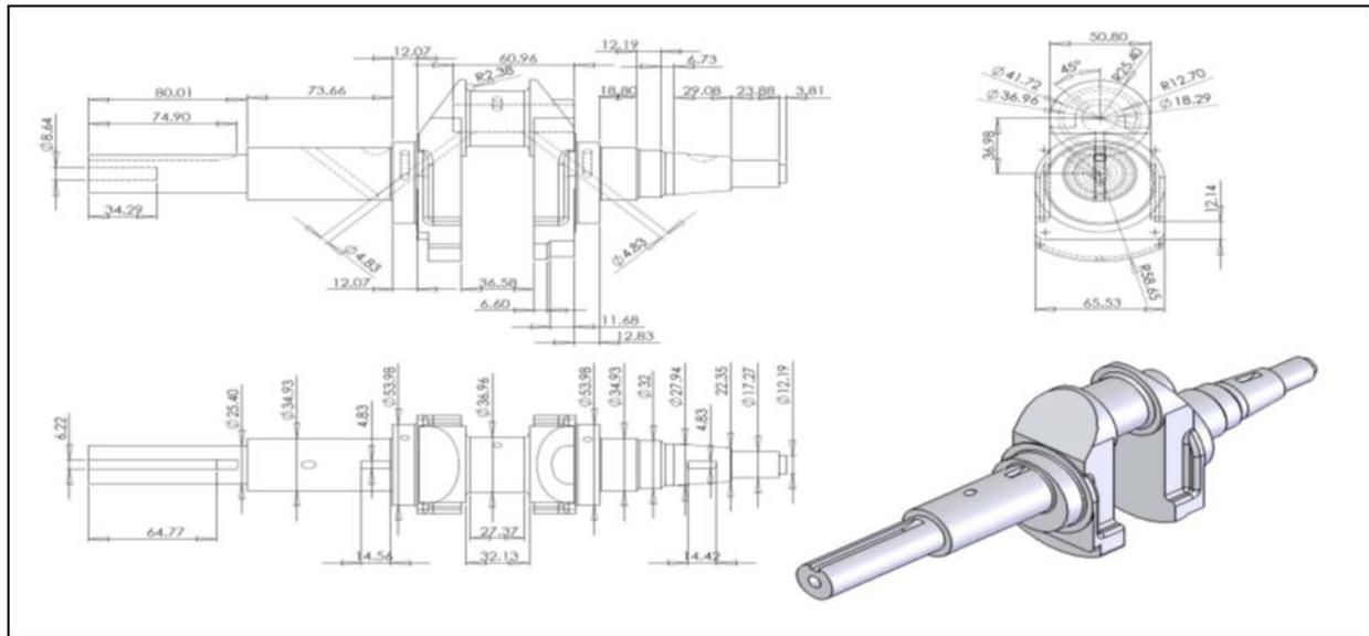
Fig 2: Dimensions of Crankshaft and 3D Model.
