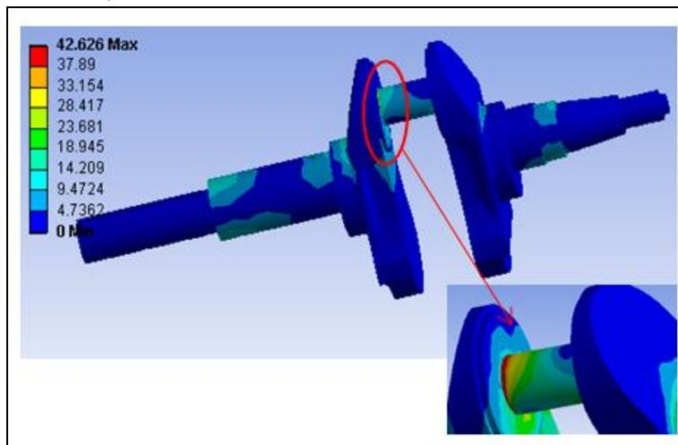
Fig 6: Maximum von-Mises Stress Plot Obtained from Harmonic Analysis for Baseline Design.
