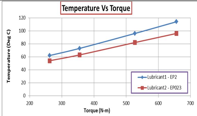
Fig 8: Temperature versus Torque Plot for both the Lubricants.
