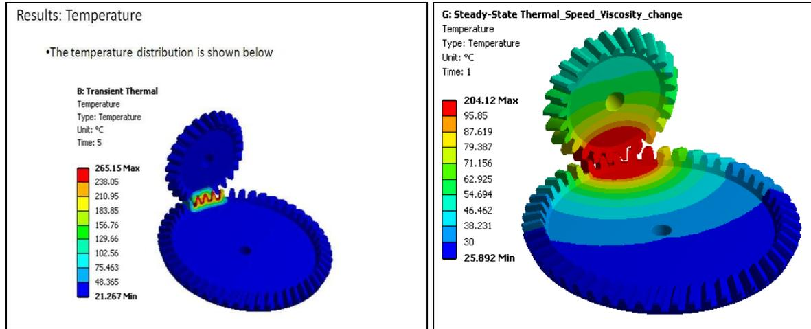
Fig 6: Thermal Analysis of Gear and Pinion.
