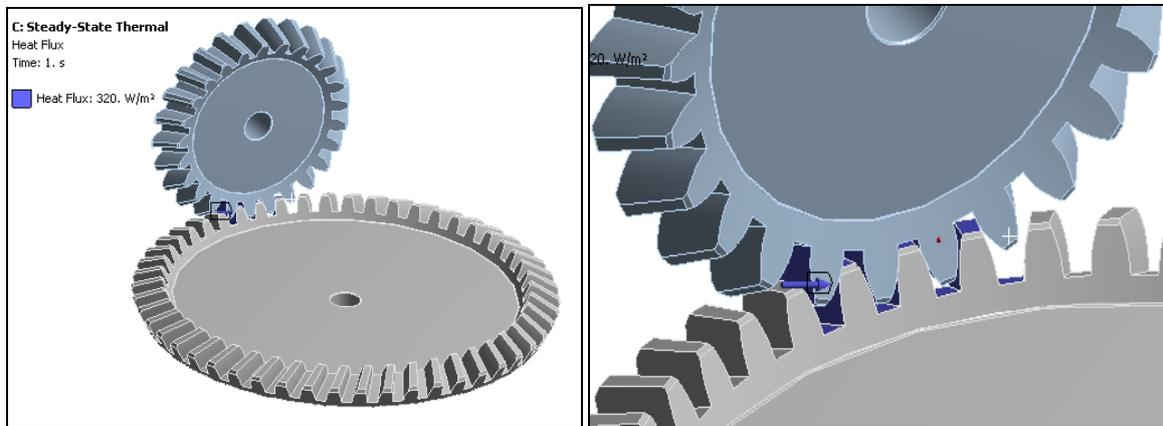
Fig 4: Plot Showing Heat Flux at the Contact Region.
