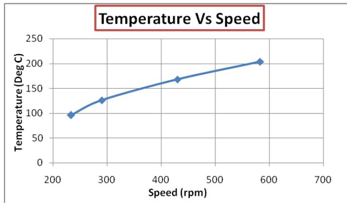
Fig 7: Temperature Versus Speed Plot Obtained from Ansys.
