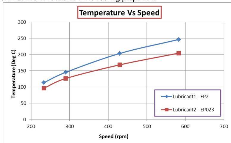
Fig 9: Temperature versus Speed Plot for both the Lubricants.
