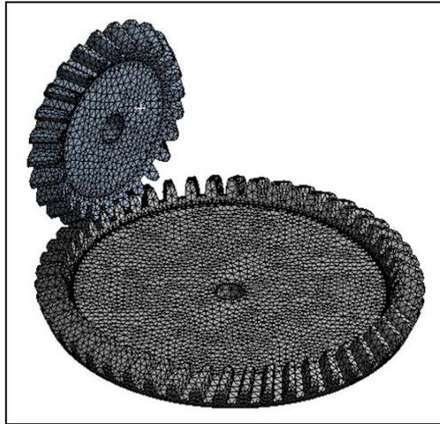
Fig 3: Mesh Model of Gear Train.
