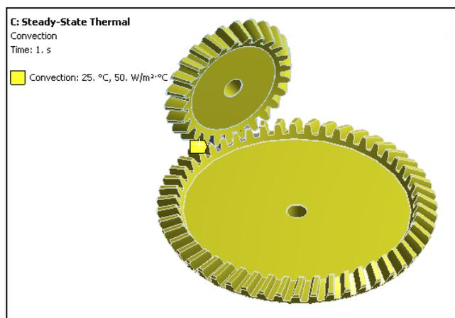
Fig 5: Plot Showing Free Convection Applied on the Gear Assembly.
